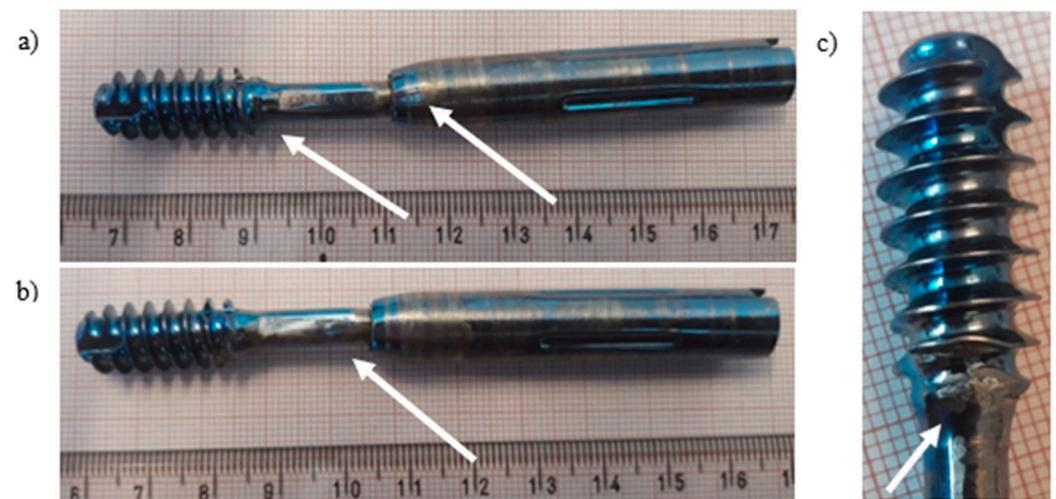
**Figure 10.** Visual inspection of the exploited telescopic lag screw (number 7 in Figure 9b) of the titanium implant: multiple cracks found on both sides of the telescopic lag screw (a,b); broken thread (c).
