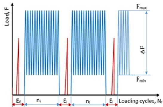
Fig. 1. Schematic illustration of the loading sequences.
