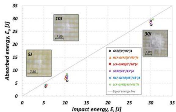
Fig. 3. EPD used in analysis of the effect of fatigue aging on the penetration threshold of the all tested GFRE.
