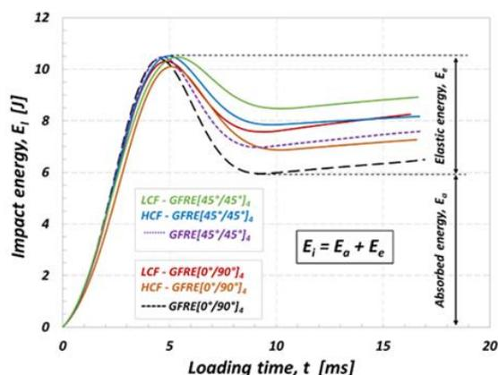
Fig. 2. Effect of fatigue aging on the  $E_a$  of the non-aged and aged GFRE for impact energy equal to 10 J.
