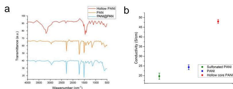
Figure 2. a) ATR-FTIR spectra of hollow PANI, PAN, and PANI@PAN. b) Conductivity of different types of PANI
