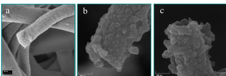
Figure 1. FE-SEM microscope conducted on nanofibers of a) PAN, b) PANI@PAN and c) hollow core PANI. The cross-sections of the hollow nanofibers clearly show their hollowness.
