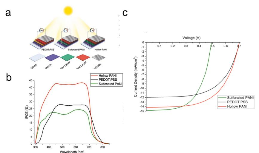
Figure 3. a) Schematic of the manufactured solar cells b) IPCE spectra of the polymer solar cells fabricated using PANI, PEDOT:PSS and hollow core PANI as buffer layers c) Performance of synthesized buffer layers via J-V characterization of different polymer solar
