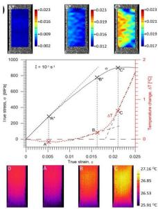
Based on the obtained mechanical and thermal characteristics, the subsequent stages for the Gum Metal loading can be distinguished:  $0 - A^*$ ; elastic deformation stage, accompanied by drop in temperature, like for other solid materials,
