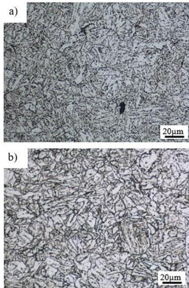
**Fig.3.** The microstructure of P91 steel in as-received condition (a) and after 80 000 h of exploitation (b).
