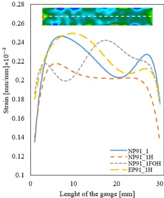
Fig. 6. Strain profiles across the gauge length.
