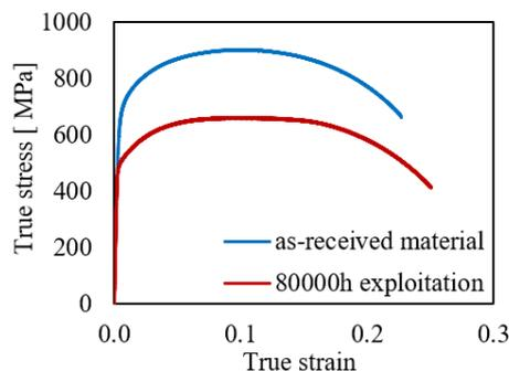
**Fig.4.** Tensile characteristics of P91 steel.
