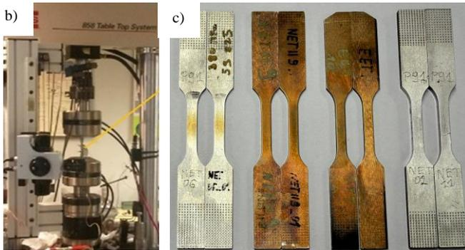
**Fig.1.** Experimental details: (a) engineering drawing of specimen for fatigue tests; (b) experimental setup showing position of the ESPI apparatus; (c) general view of the tested specimens.
