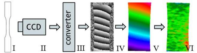
**Fig.2.** The experimental procedure of ESPI measurement: recording of interference results from the specimen surface (I) as speckled images using the CCD camera (II) and converter (III); generation of correlation fringes through the subtraction process of obtained speckle interferograms (IV); determination of a phase map presenting the distribution of displacement and average strain components in each direction separately (V) and the field stress and strain phase maps (VI).
