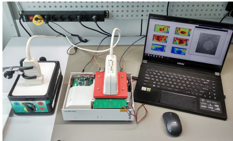
Figure 6. The setup that was used in this work. Left to right: the L7-4 probe over the CIRS 049A elastography phantom, the us4R-lite portable research platform with the TX extension board mounted and connected to the PC with Mathworks MATLAB software running.
