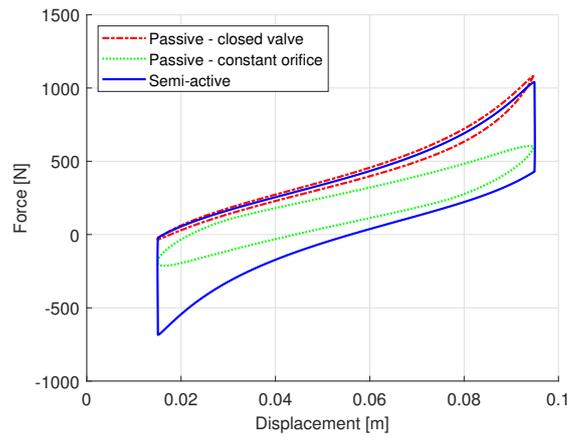
Figure 4: Numerical model response in displacement domain in three modes of operation
