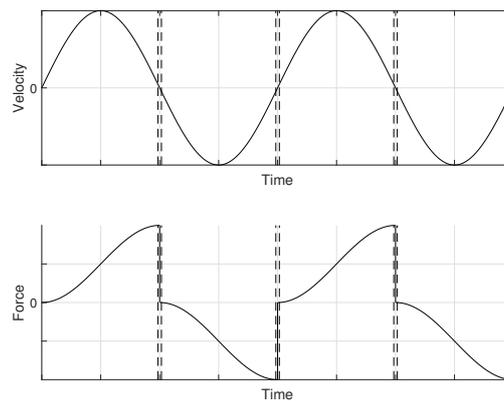
Figure 2: An illustration of the semi-active system operation under a harmonic excitation. Switching instants are depicted with dash lines
