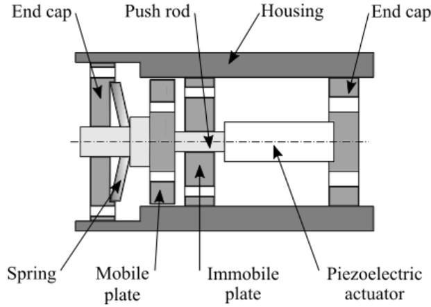
Figure 1: High performance valve - scheme.
