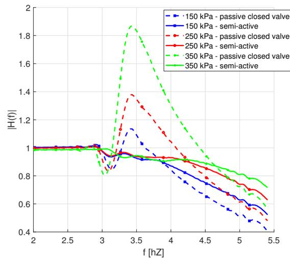
Figure 8: Transfer Functions of the PAA absorber on a 1DoF kinematic vibration test stand. Suspended mass 27 kg. Comparison of passive and controlled responses of the system with a variety of the initial pressures.
