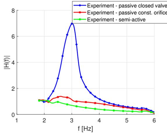
Figure 6: Experimentally obtained Transfer Functions of the system in three modes of operation: passive with continuously closed valve, passive with constant orifice, semi-active.
