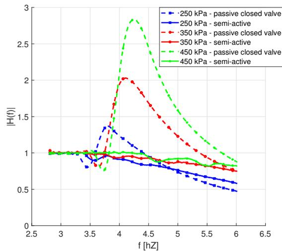
Figure 7: Transfer Functions of the PAA absorber on a 1DoF kinematic vibration test stand. Suspended mass 17 kg. Comparison of passive and controlled responses of the system with a variety of the initial pressures.
