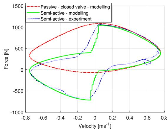
Figure 5: Numerical model versus experimental response in velocity domain
