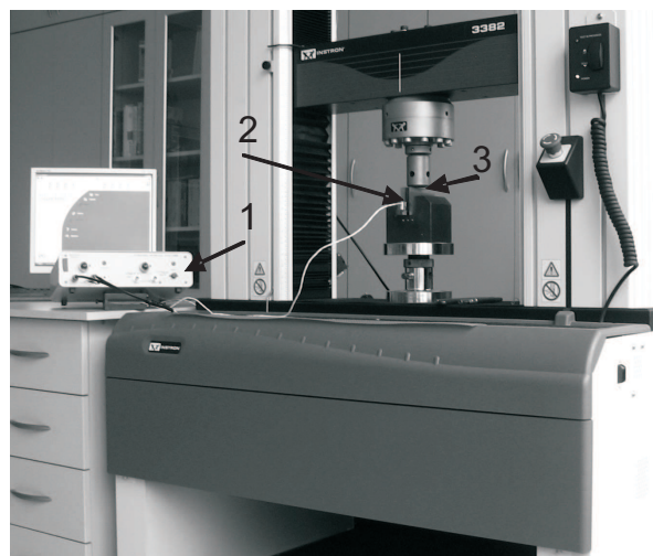
Fig. 1. Two-channel measuring system applied to mechanoacoustic tests of the ceramic samples. There are marked: 1 – AE analyser, 2 – acoustic transducer, 3 – enclosure containing the sample
