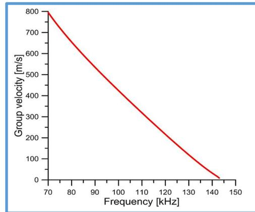
Fig. 4. Group velocity of the new torsional elastic wave versus frequency.
