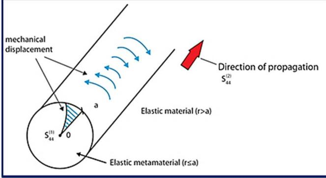
Fig. 1. Cross-section of the waveguide supporting the newly discovered torsional elastic surface waves, propagating in the direction along the cylindrical metamaterial rod ( $r < a$ ) embedded in a conventional elastic half-space ( $r > a$ ). Mechanical displacement  $u_\theta$  of the new torsional elastic surface waves is polarized along the angular coordinate  $\theta$ . The radius of the inner metamaterial rod is assumed to be 1 cm.
