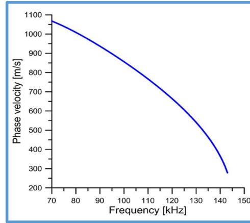
Fig. 3. Phase velocity of the new torsional elastic wave versus frequency.
