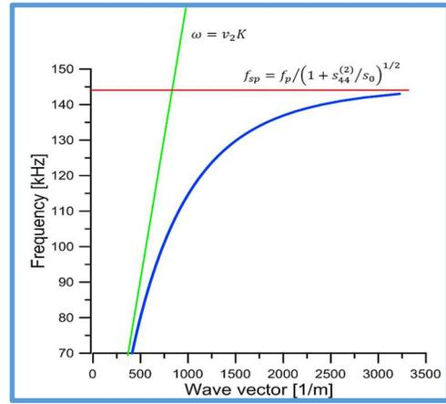
Fig. 2. Dispersion curve ( $f$  versus  $K$ ) of new torsional elastic surface waves.
