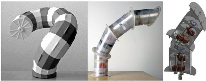
**Fig. 3** Left: 3D-printed mock-up of a dodecagonal 12 module Arm-Z. Middle: An early prototype of a 4-unit Arm-Z. Right: Isometric cutaway showing the drive for rotation which is carried by the gear system.
