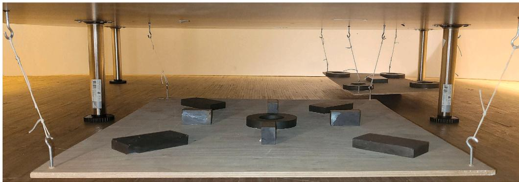
Fig. 4. System for creating magnetic field on the test stand.
