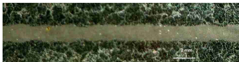
Fig. 3 – Oscillations of the fusion zone in the cross section parallel to the facing surface (AZ91 joint, cross section made at 1.5 mm from the face surface).
