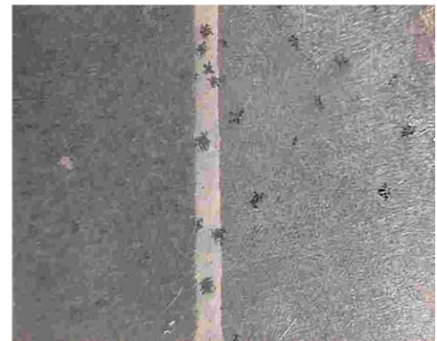
Fig. 14 – The surfaces of the joints and the surroundings after corrosion tests.
