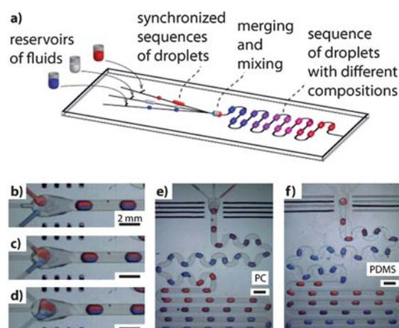
**Fig. 2** (a) A schematic illustration of the integrated system for high-throughput scanning of reaction conditions. Three consecutive micrographs (b) through (d) recorded at 125 fps, show the process of merging of droplets into the reaction mixtures. Insets (e) and (f) illustrate sequences of concentrations formed in chips fabricated in PC and PDMS.
