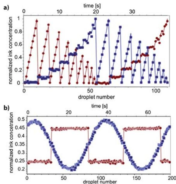
**Fig. 3** The graphs show two sequences of concentrations of the reaction mixtures formed in the integrated systems (lines show expected concentrations, while symbols correspond to the values measured experimentally).
