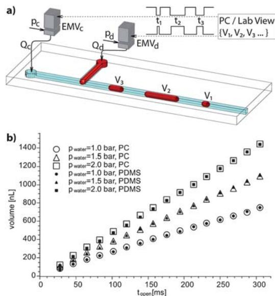
**Fig. 1** (a) A schematic illustration of the DOD system with two electromagnetic valves controlling the flow of the continuous fluid (drawn from a reservoir maintained at a pressure  $p_c$ ) and the droplet phase ( $p_d$ ). (b) Volumes of the droplets generated by this system connected to polycarbonate (PC) or polydimethylsiloxane (PDMS) chips. The cross-section of the channels was  $400 \mu\text{m} \times 400 \mu\text{m}$ . Droplets generated at 3 Hz,  $p_{oil} = 0.4$ .
