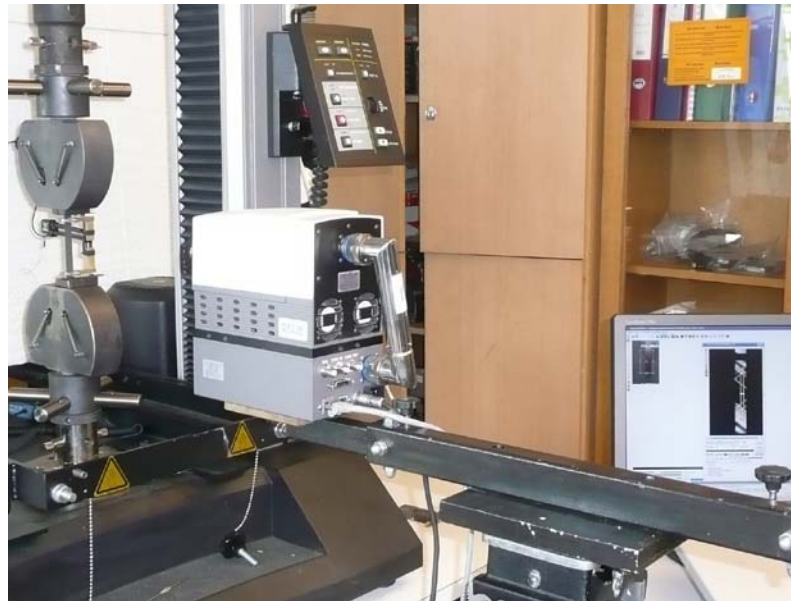
Fig. 1. Photograph of TiNi SMA specimen with mechanical extensometer in grips of Instron testing machine, Flir Phoenix infrared camera and temperature distribution image of localized martensite transformation
