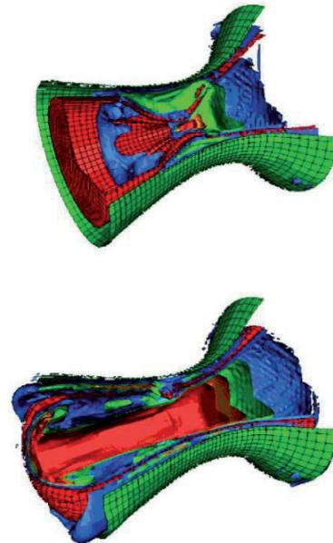
**Fig. 6:** ALE FSI model of the HPV closing sequence
