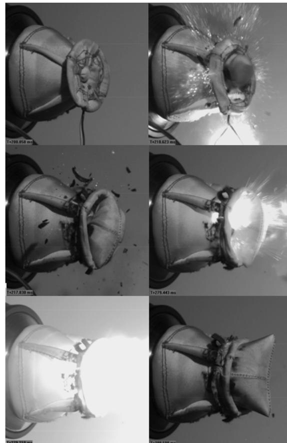
**Fig. 7:** HPV closing sequence
