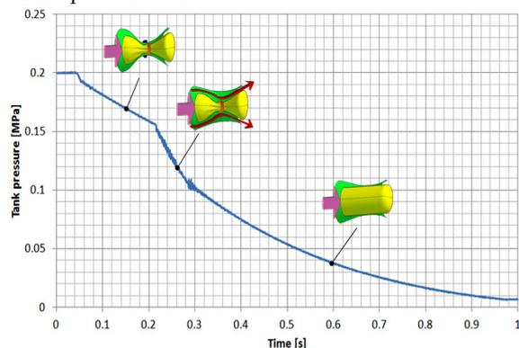
**Fig. 8:** Test tank internal pressure as a function of time
