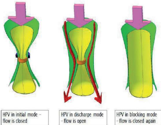
**Fig. 5:** HPV operation sequence
