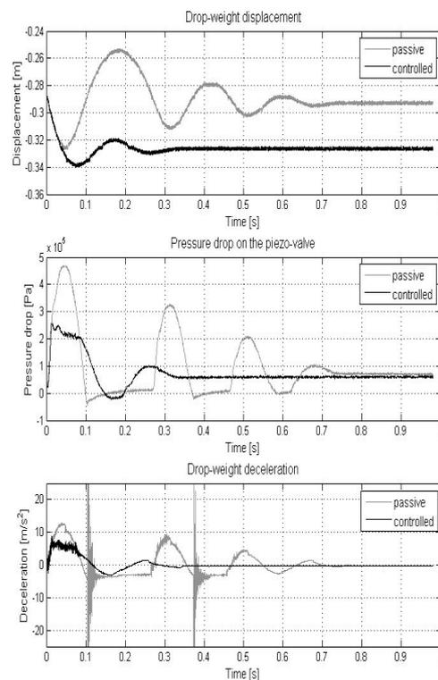
Fig. 4: HPA performance under impact loading
