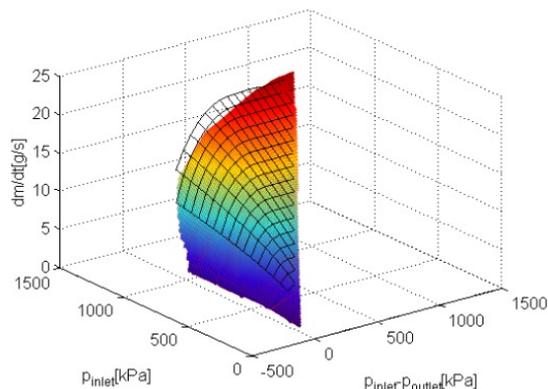
Fig. 3: HPA piezo-valve performance
