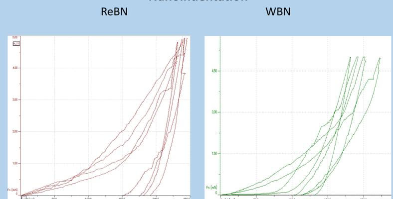
Results of Vickers hardness of ReBN sample (a) 5685.6 MPa and WBN sample (b) 9004.3 MPa,
