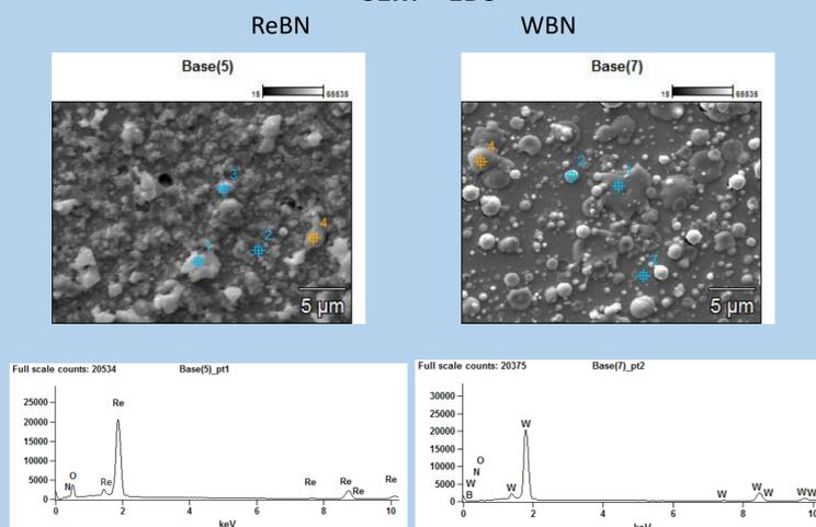
ReBN and WBN layers were characterized by low nitrogen content. The ReBN layers have low density and irregular structures on the layers surface. The WBN layers are dense but are composed mainly by droplets.
