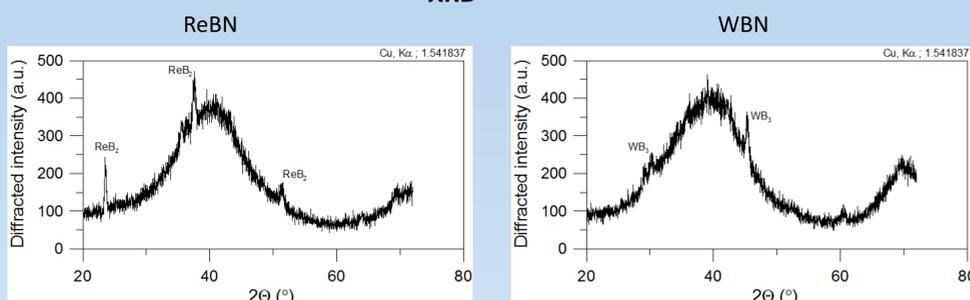
ReBN and WBN coatings are amorphous. XRD diffractogram contain only a single peaks from the crystalline phase.
