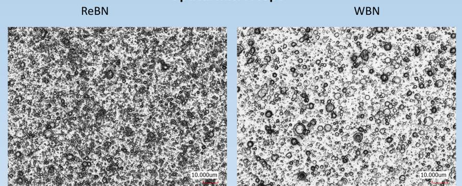
The thickness of RF-PLD layers: ReBN  $\sim 2 \mu m$ , WBN  $\sim 2 \mu m$ . Layers are characterized by high roughness but no delamination were observed.
