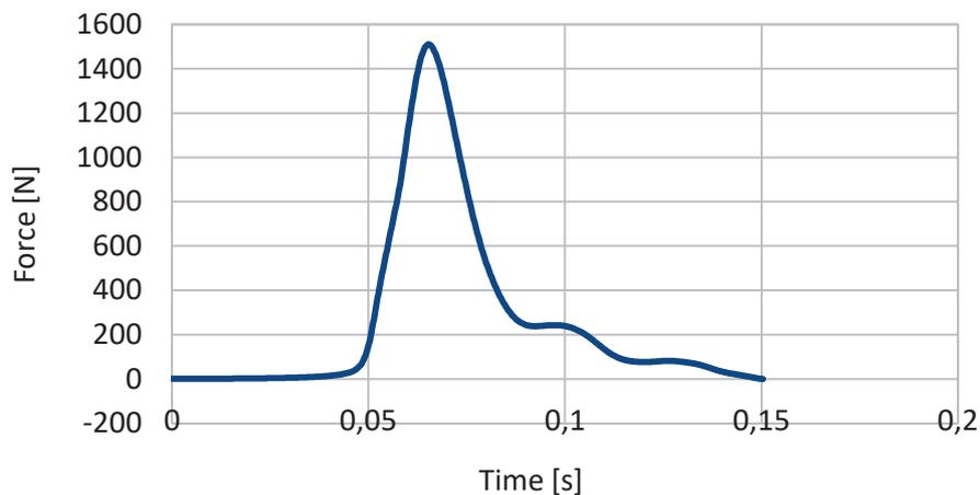
Figure 7: Interface force of the airbag in time domain
