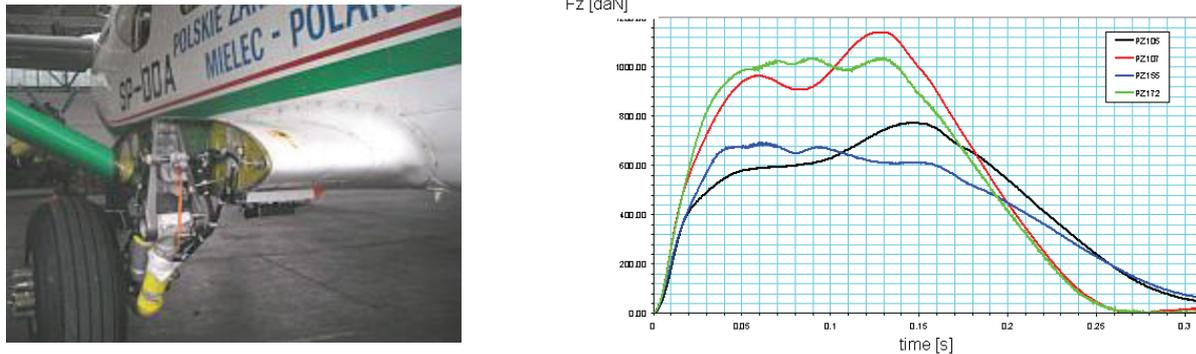
Figure 1: Adaptive aircraft landing gear (FP7 project ADLAND - flight tests, experimental results)
