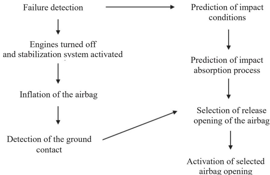
Figure 4: The general scheme of emergency system operation
