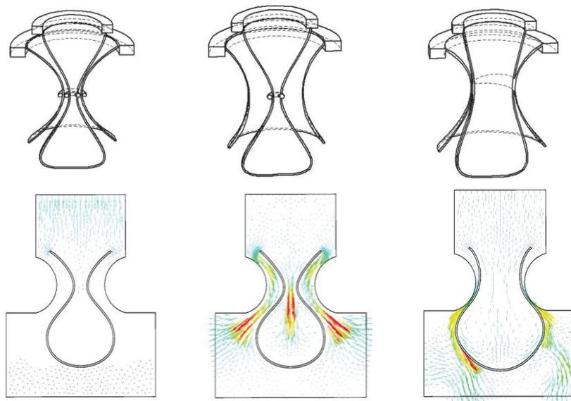
Figure 3: The cross-section of the membrane valve and simulation of the gas flow during subsequent stages of valve operation.
