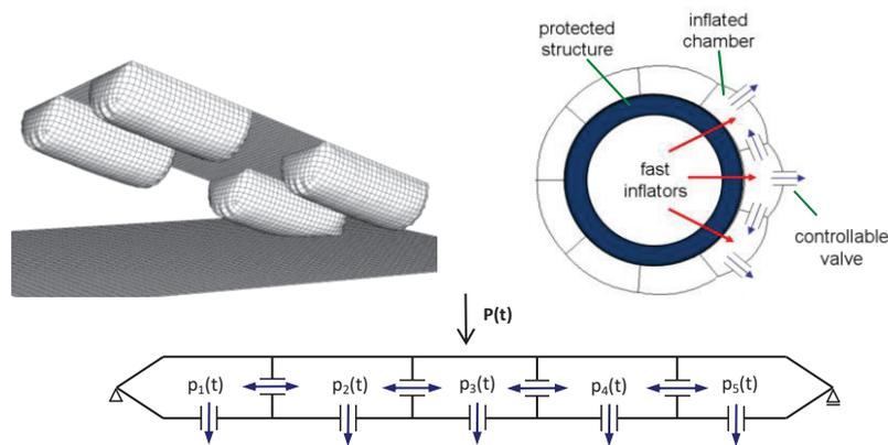
Figure 2: Adaptive Inflatable Structures: a) emergency flow control-based airbags, b) inflatable fenders, c) adaptive inflatable barrier
