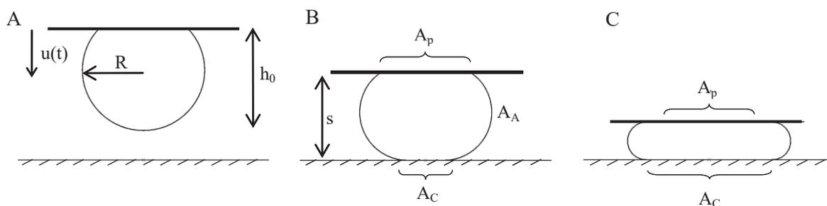
Figure 5: Three stages of the process of landing with adaptive airbag
