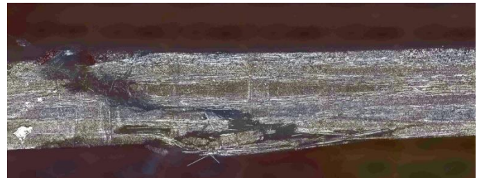
Fig. 3. Microscopic image of the structure of the sample „+” with the highest compressive strength
