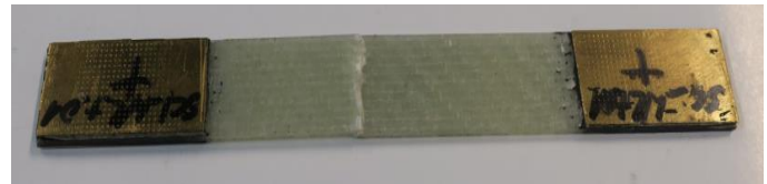
Fig. 2. The shape of the sample „+” subjected to the compression test
