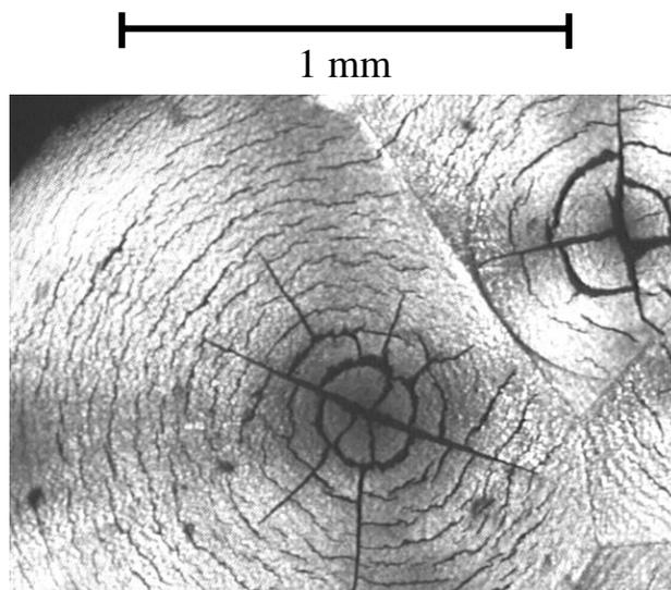
Figure 3. Optical micrograph (crossed polars) of PHB film, crystallized during cooling at 5°C/min, after melting at 200°C for 3 min.
