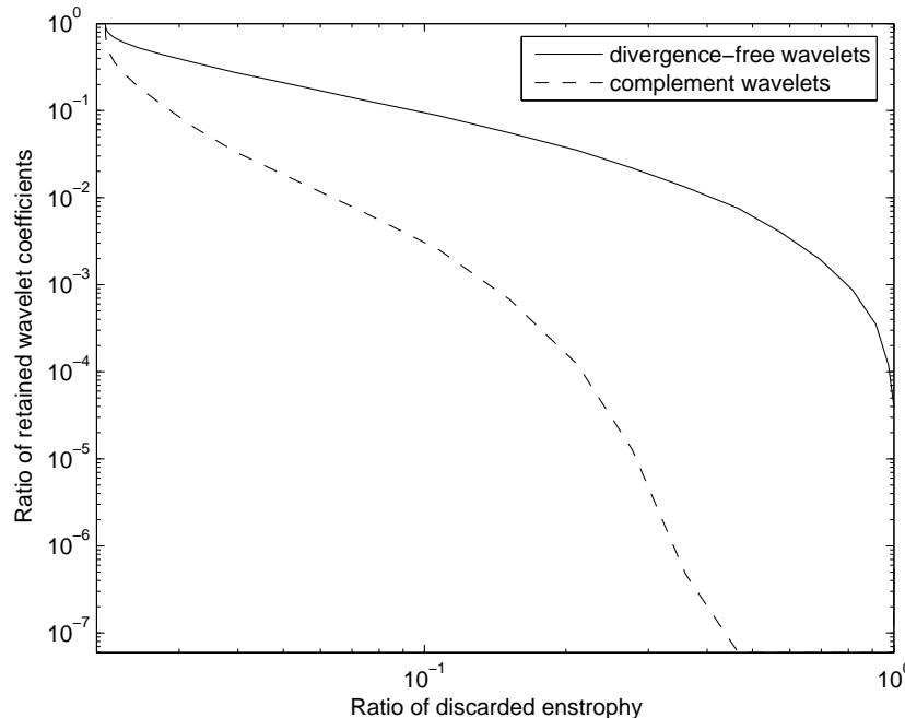
*On the left, comparison between isotropic and anisotropic div-free wavelet compression in semi-log scale. On the right, contributions from div-free coefficients and complement coefficients.*
