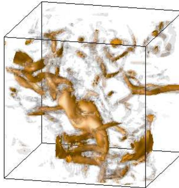
*A sub-cube  $64^3$  of the initial turbulent field  $256^3$  ( $Re=260$ )*
