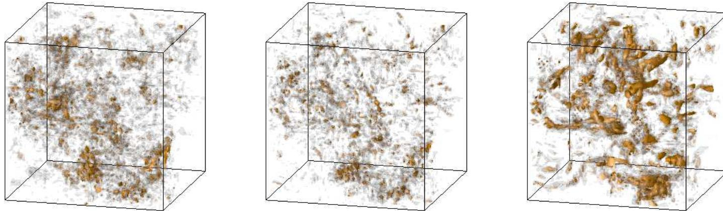
*Incoherent part with the div-free wavelets (left), the orthogonal Coifman 12 wavelets (center) and the biorthogonal Harten wavelets (right).*
