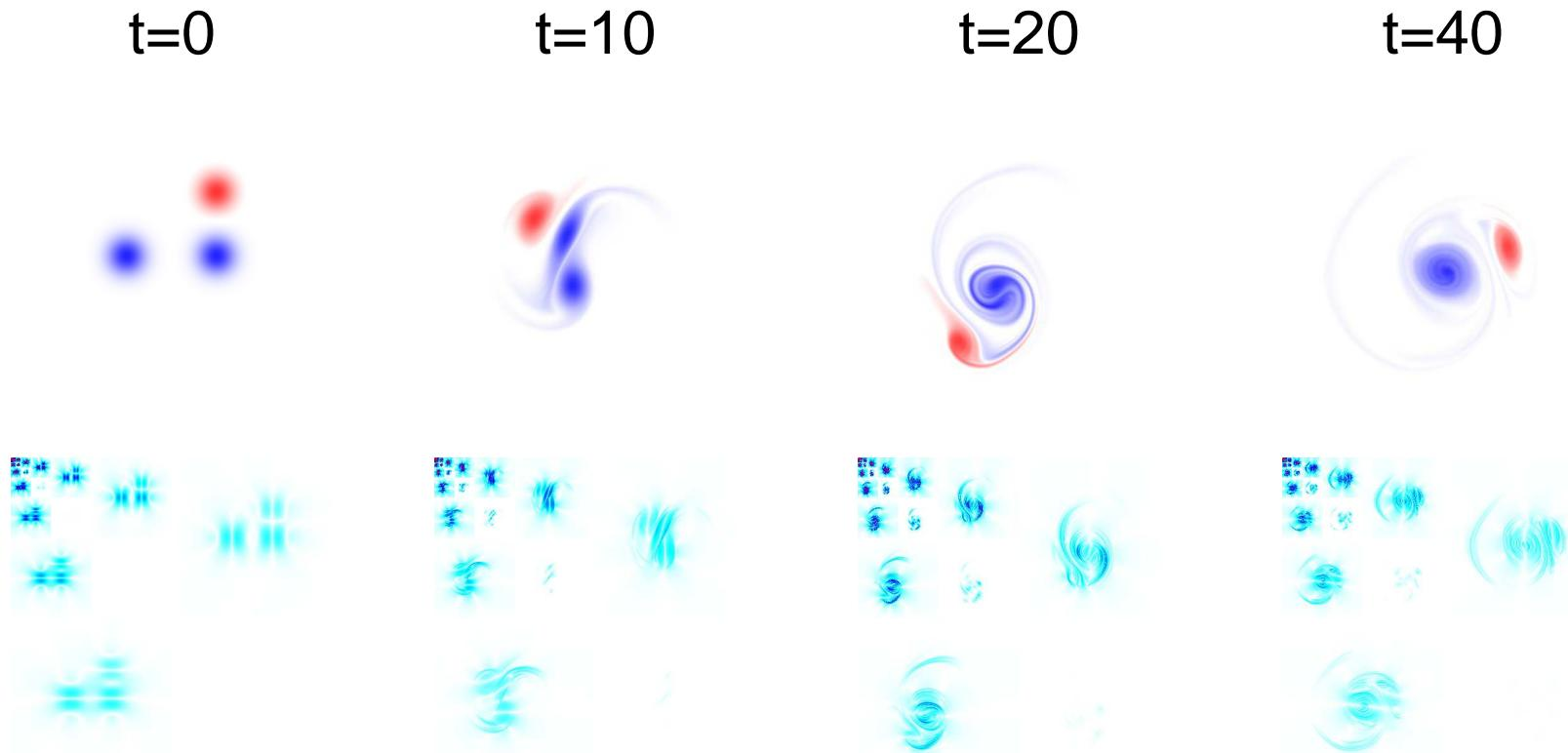
Vorticity fields and wavelet coefficients on a  $512^2$  grid,
