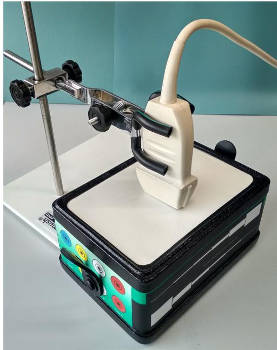
**Figure 1:** The QA elasticity phantom in a test setup with probe.
