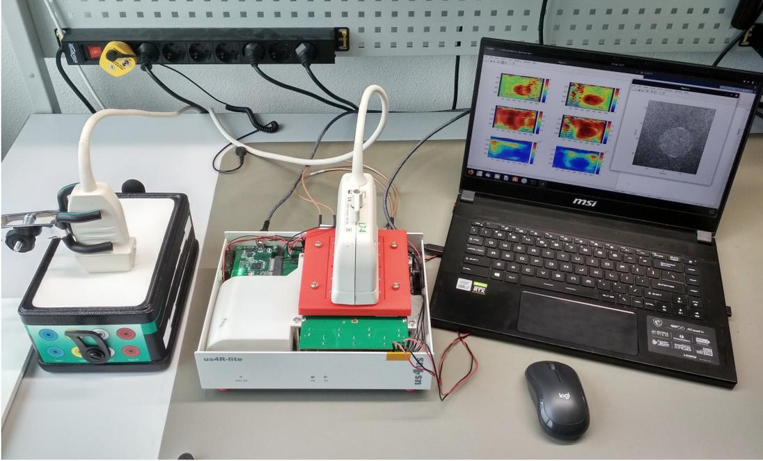
**Figure 4.5:** The setup that was used in this work. Left to right: the L7-4 probe over the CIRS 049A elastography phantom, the us4R-lite portable research platform with the TX extension board mounted and connected to the PC.
