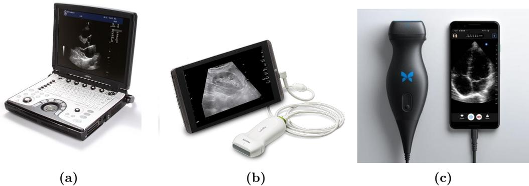
**Figure 1.1:** Various point-of-care ultrasound systems: (a) GE Logic e (General Electric, Boston, USA) in a form of a compact laptop. (b) Philips Lumify (Philips, Amsterdam, The Netherlands) with front-end electronics integrated within the probe. (c) Butterfly iQ+ (Butterfly Network, Guilford, USA) — a complete solution in a single probe that can be connected to a mobile phone. It utilizes a CMUT (capacitive micromachined ultrasound transducer) with over 9000 elements [11]
