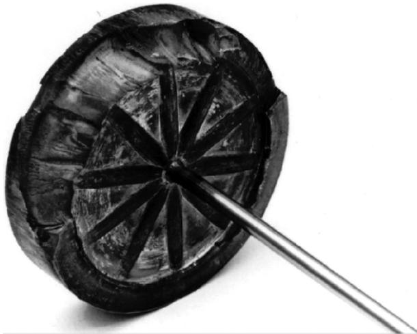
**Figure 1.3** The pattern of the aluminium rest and extruded wire. The extrusion ratio equals 700. *Source:* Korbel and Szyndler 2010. Copyright of Włodzimierz Bochniak.
