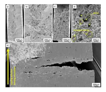
Fatigue Damage Evolution in SS316L Produced by Powder Bed Fusion in Different Orientations with Reused Powder Feedstock
