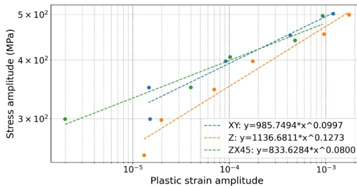
Fig. 1 Cyclic stress – strain curves for three orientations of specimen's axis in AM
