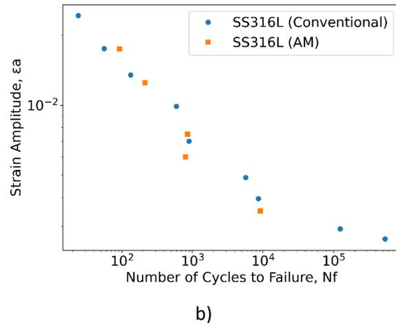
Fig. 2 LCF results of SS316L: a) CSS curves, b) e-N curves, c) DIC technique applied on specimen manufactured by AM
