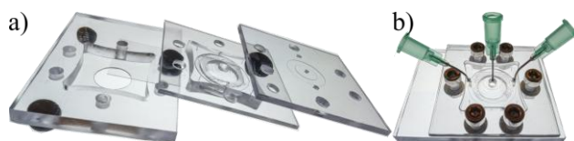
Fig.1. The microfluidic chip. (a) The microfluidic device consists of several layers of polycarbonate that are connected using thin PDMS gaskets. The cells are grown on a microscope cover glass. (b) The chip's appearance after assembly.
