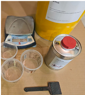
Fig. 2. Poured polymer sheets and PS adhesive components prepared for mixing.
