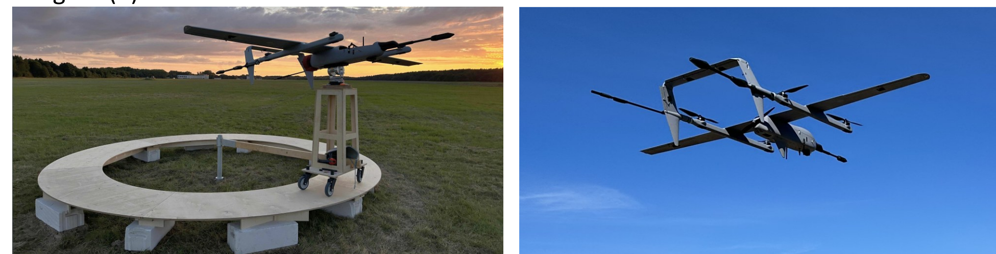
Fig. 2. Calibration stand for the tail-mounted scalar magnetometer. The stand enables systematic data collection across the UAV's operational attitude range while maintaining the magnetometer in a fixed position, which isolates it from local magnetic anomalies (l.h.s.), VTOL platform with a tail-mounted magnetometer for magnetic field mapping and formation-flight data simulation (r.h.s.).
