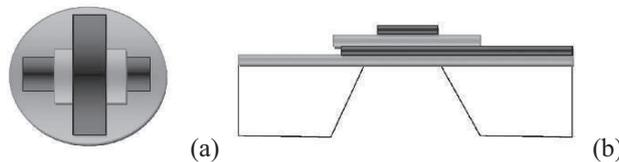
Fig. 1. The resonator, top view (a), cross-section (b)
