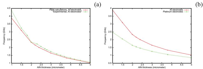
Fig. 3. Numerical results and experimental results for Al electrodes (a), numerical results for Al and Pt electrodes (b)
