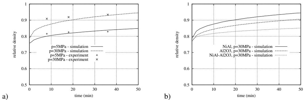
**Rysunek 2.** Evolution of relative density during sintering: a) numerical vs. numerical results for NiAl, b) numerical results for NiAl, Al<sub>2</sub>O<sub>3</sub> and mixture NiAl/Al<sub>2</sub>O<sub>3</sub>.
