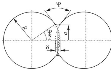
**Rysunek 1.** Two-particle model of sintering.
