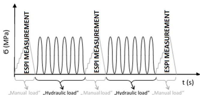
Fig. 3 Scheme of loading during the interrupted fatigue test.
