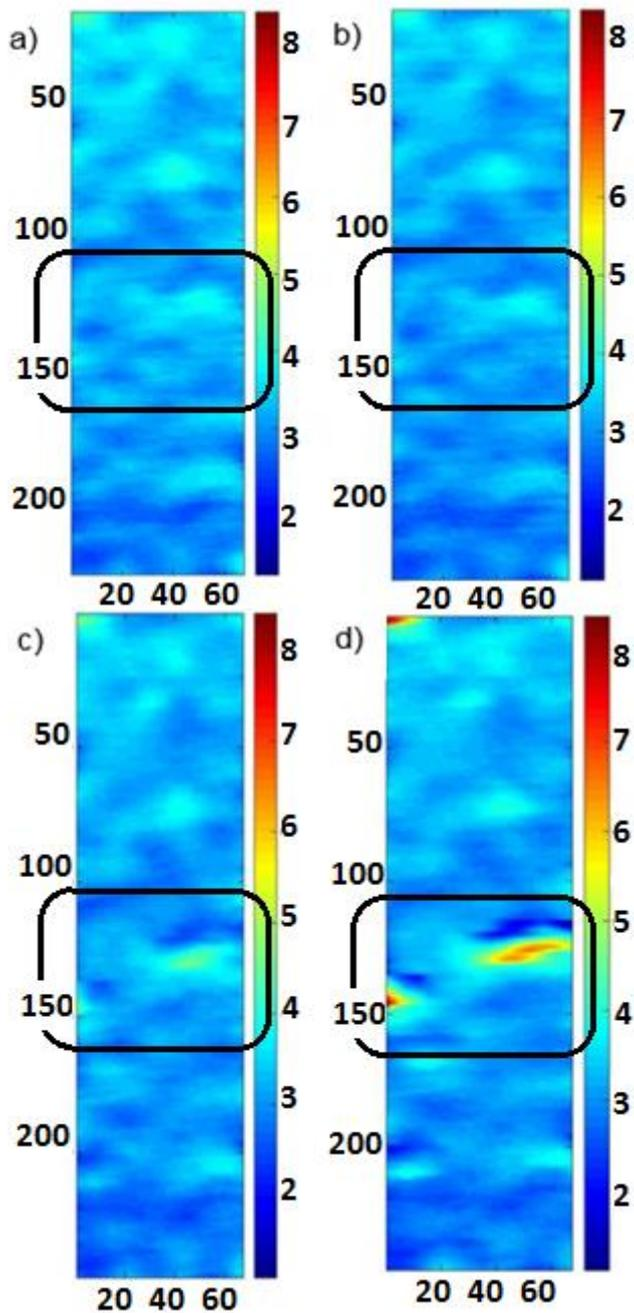
Fig. 5. The full-field strain distributions along Y axis corresponding to the stress direction. Measurements are performed: (a) during the first cycle, (b) after 20000 cycles, (c) after 40000 cycles, (d) after 50000 cycles. The scale is matched to the extreme strain magnitudes of all measurements:  $\epsilon_{MIN}=1,1 \cdot 10^{-3}$ ,  $\epsilon_{MAX}=8,4 \cdot 10^{-3}$ .
