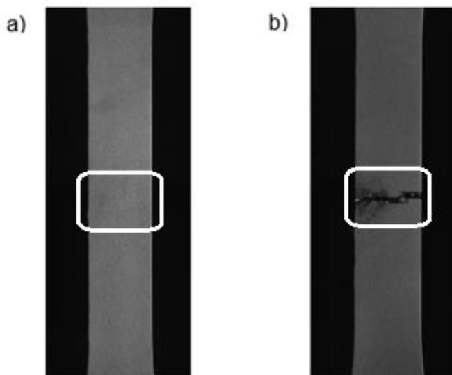
Fig. 7. Fatigue specimen photo: (a) before fatigue test; (b) after fatigue test ( $N_f=54315$  cycle)
