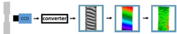
Fig.1. Scheme of subsequent steps during ESPI measurement [1]
