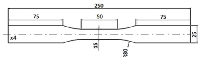
Fig.2. Geometry and dimensions of the fatigue specimen.
