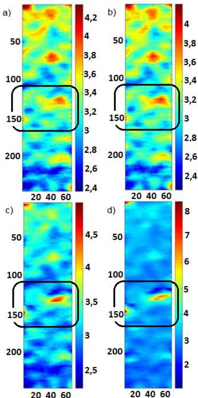
Fig. 4. The full-field strain distributions along Y axis corresponding to the stress direction. Measurements are performed: (a) during the first cycle, b) after 20000 cycles, c) after 40000 cycles, d) after 50000 cycles. The scale was automatically adjusted to the extreme strain value in each measurement.
