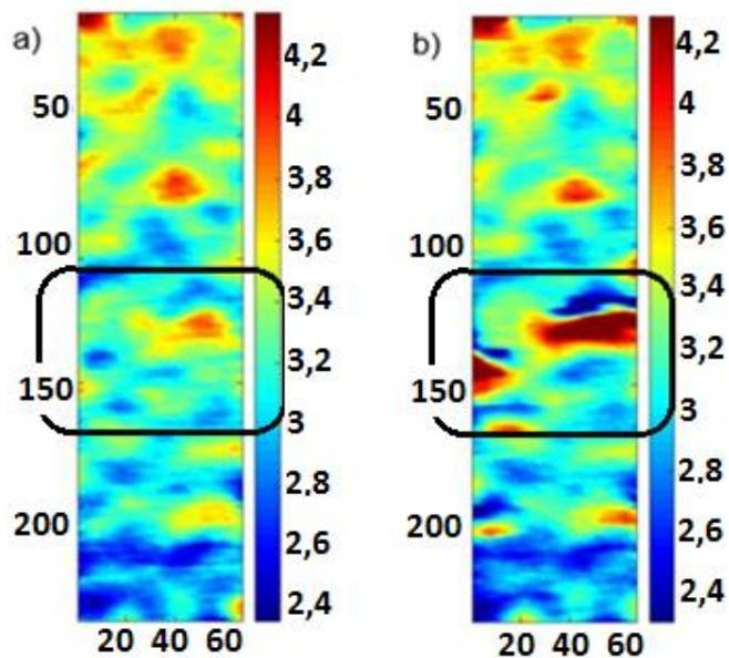
Fig. 6. The field strain distribution along Y axis corresponding to the acting stress direction. Measurements performed: (a) in the first loading cycle; (b) after 50000 cycles. Scale is matched to the extreme strain values in the first measurement.
