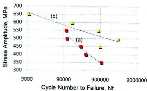
Fig. 3 Wöhler curves for Inconel 740 nickel alloy: (a) as-received, (b) with a CrN+Cr<sub>2</sub>Ni<sub>3</sub> layer.
