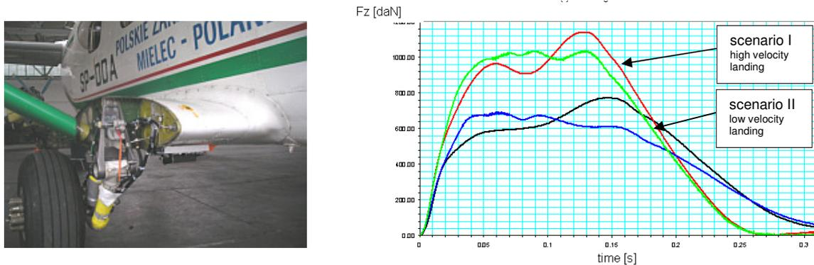
Figure 1: Adaptive aircraft landing gear - FP6 project ADLAND - flight tests, experimental results
