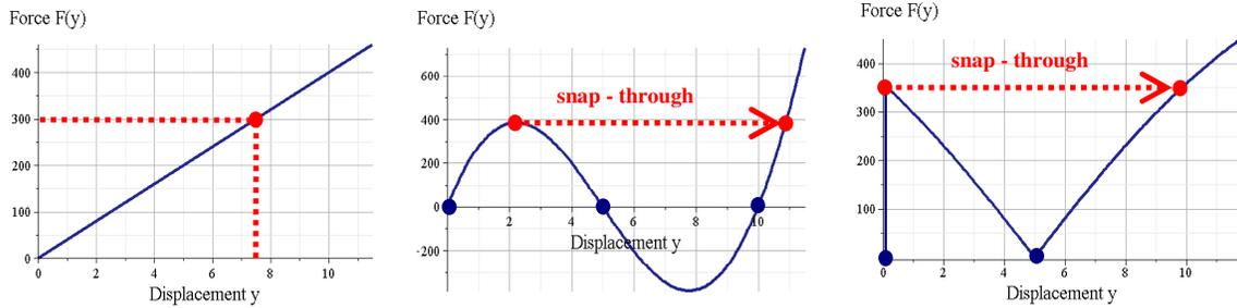
Figure 4: Comparison of dynamic characteristics of 1DOF linear system with elastic and plastic von Mises trusses
