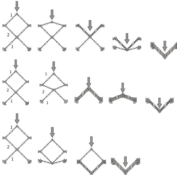
Figure 6: Folding modes for the basic multi-folding structure
