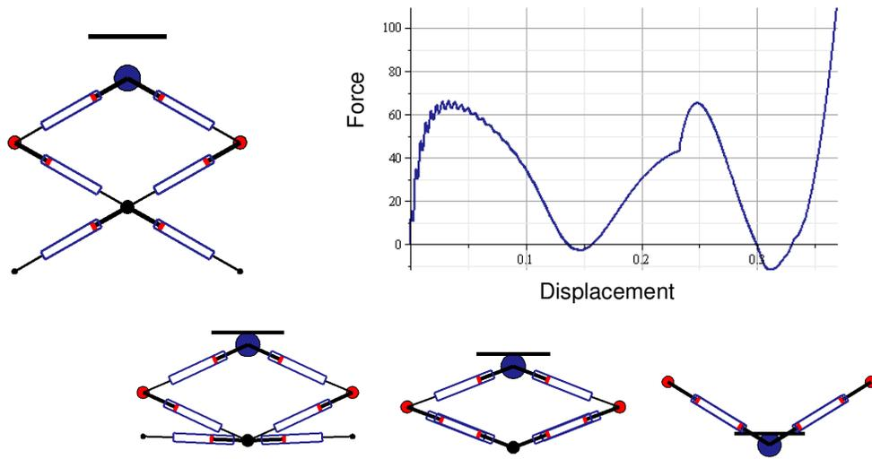
Figure 10: Force-displacement characteristics of pneumatic MFM structure
