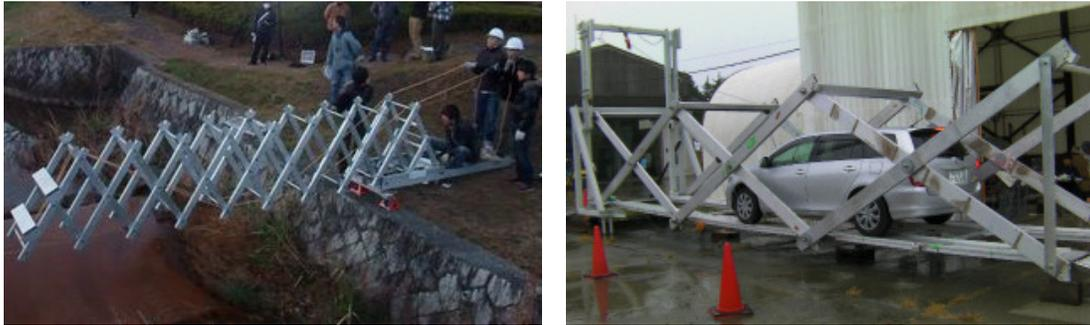
Figure 14: Applications of multifolding: to a mobile bridge
