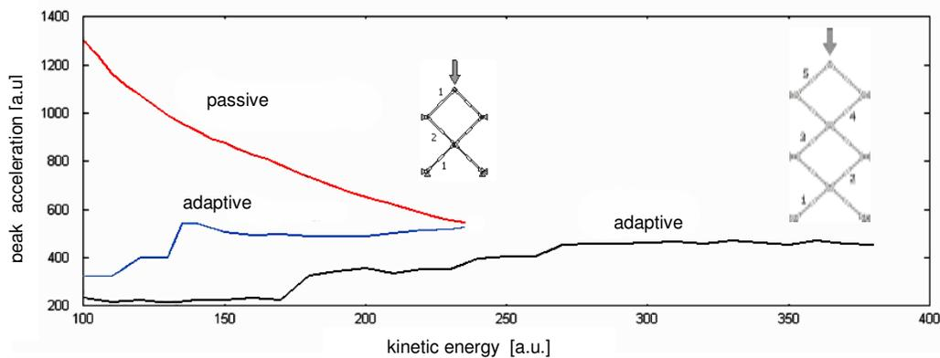
Figure 11: Comparison of the efficiency passive and adaptive multilayered MFM absorbers
