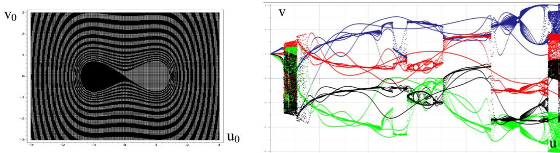
Figure 5: Response of von Mises truss to dynamic excitation: a) final location of mass in terms of initial conditions, b) response to harmonic excitation of various amplitude and phase angle
