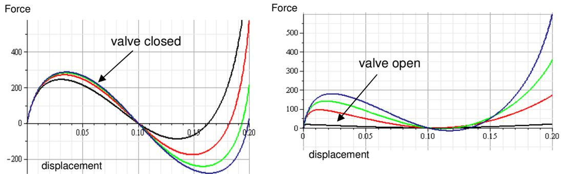
Figure 9: Force-displacement characteristics of pneumatic von Mises truss for different opening of the valve
