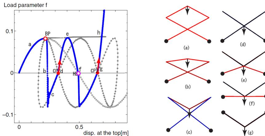
Figure 7: Equilibrium paths for the mode 1 of elastic multi-folding structure
