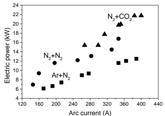
Fig.1. Input electric power for gas flow rate 0.8g/s injected into arc and 0.6g/s into plasma jet at pressure 6kPa; ■ - argon arc and nitrogen introduce into plasma jet; ● - nitrogen or ▲ - carbon dioxide introduce into plasma jet
