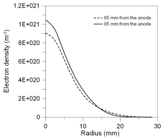
Fig. 5. Radial distributions of the electron density at two different distances from the anode
