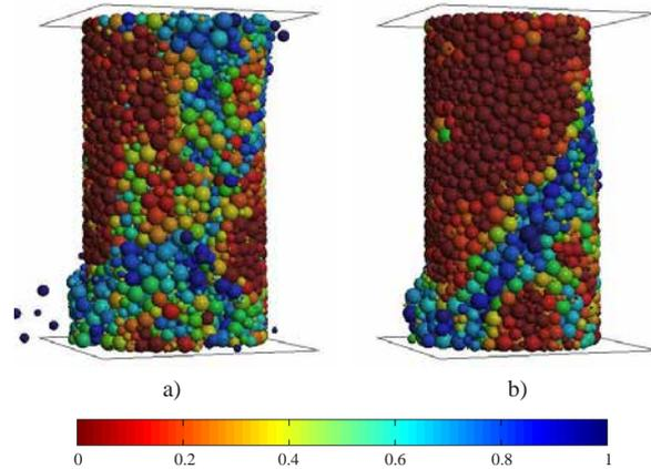
Figure 2: Fractured specimens with distribution of the damage parameter: a) model with local evaluation of the parameters, b) model with the uniform global parameters
