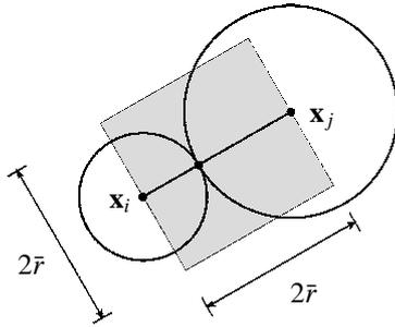
Figure 1: Schematic connection of two particles.
