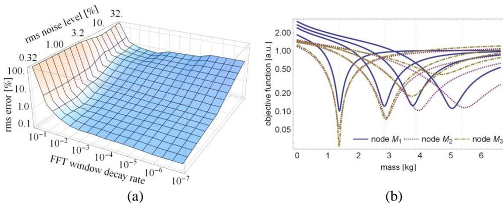
Figure 2. (a) Root mean square relative identification errors in dependence on the decay rate of the FFT exponential window and the simulated measurement noise. (b) Typical objective functions (FFT window decay rate  $10^{-5}$ , measurement noise 10% rms).
