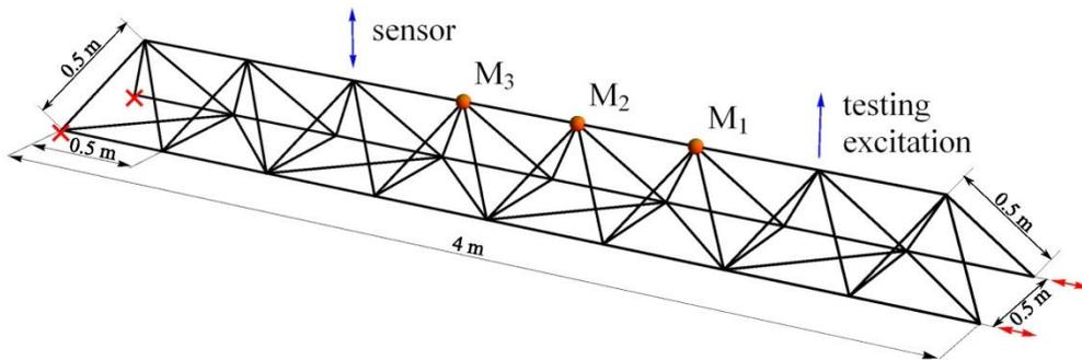
Figure 1. Truss structure used in the numerical example.
