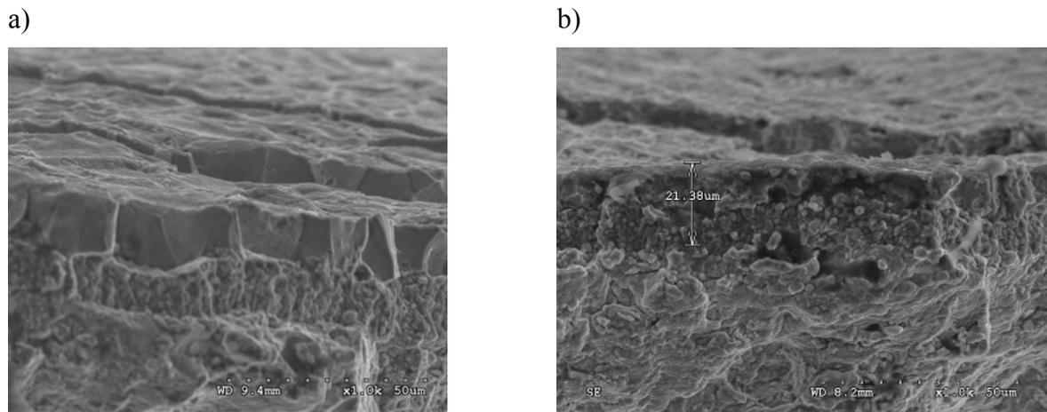
Fig. 7. Image of sample fractured sample surface, visible nickel alloy base with aluminide coating
