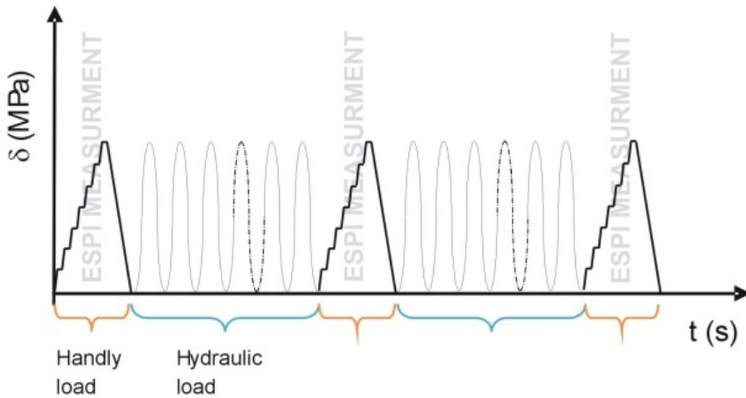
**Fig. 2** Diagram presenting sample load in fatigue cycles
