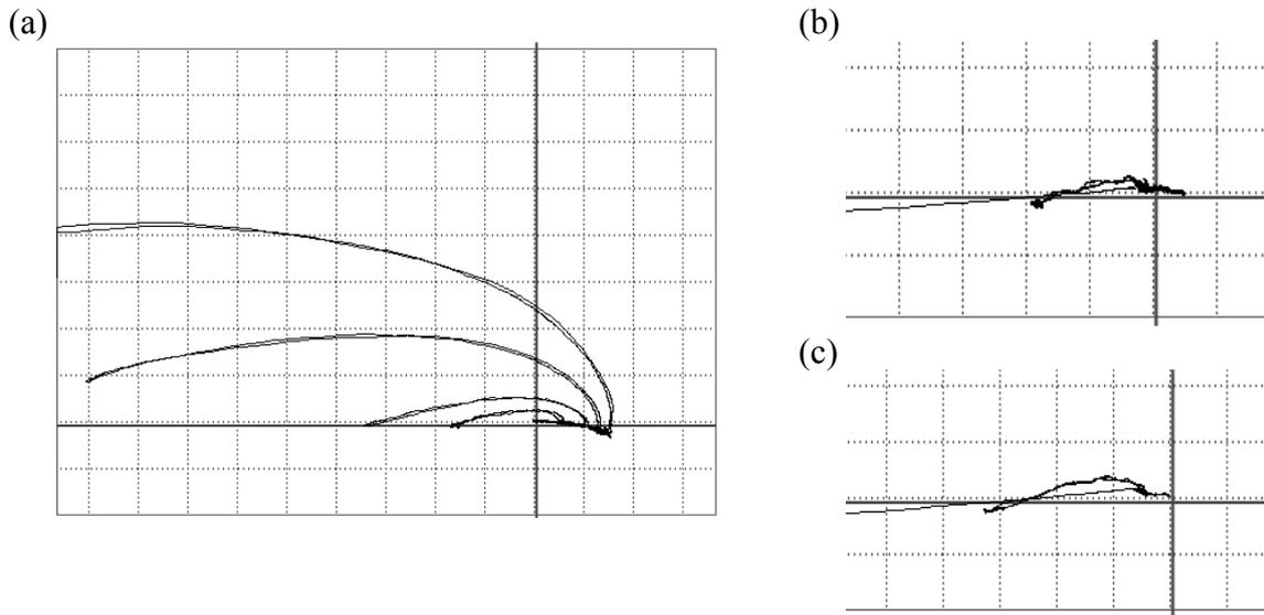
Fig. 6. ET signal changes indicated by discontinuities on the reference sample (a), in the unloaded (b) and loaded (b) sample after 50,000 cycles
