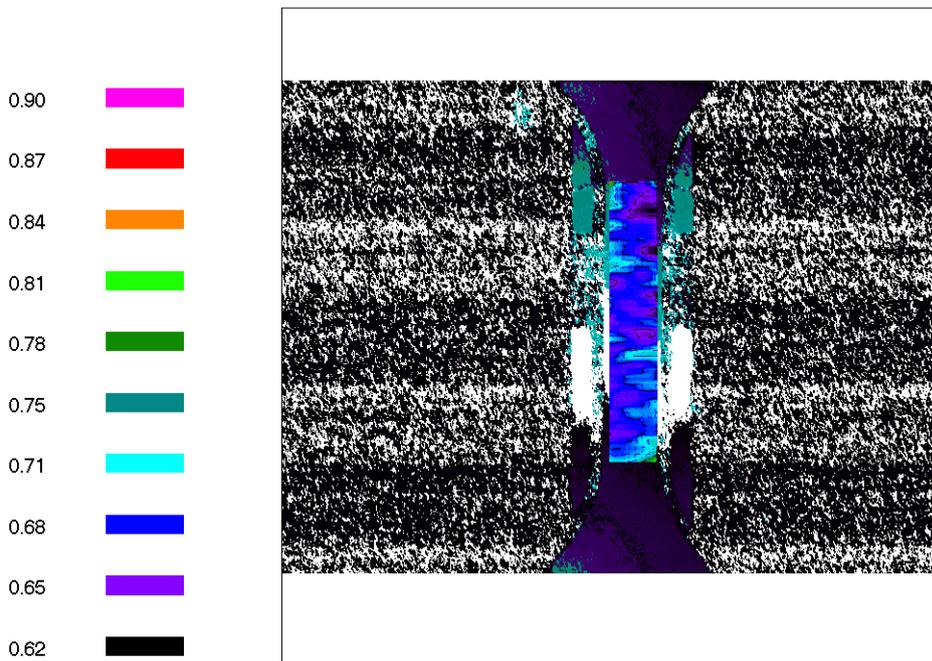
**Fig.3.** Interference image with superimposed map of specimen deformation generated by the ESPI
