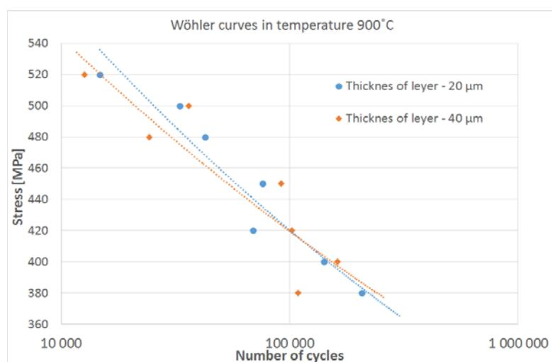
**Fig. 4.** Wöhler characteristics for specimens with surface deposited by aluminide layer
