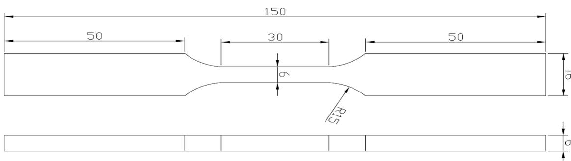
**Fig. 1.** Sample geometry for fatigue test with elongated gauge length enabling measurement of changeable eddy currents values
