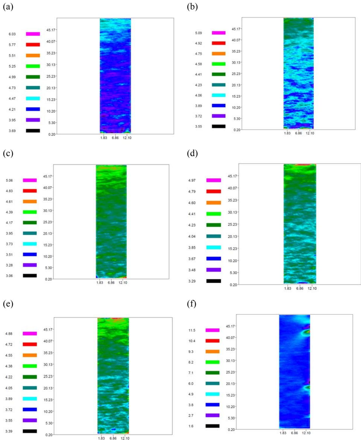
**Fig. 5. Deformation map** of sample surface for (a) 1 cycle (b) 10 001 cycle, (c) 20 001 cycle, (d) 30 001 cycle; (e) 40 001 cycle; (f) 50 001 cycle of fatigue test
