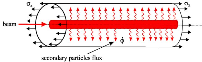
Fig. 1. Coaxial target – detector configuration (round bar and cylindrical shell)
