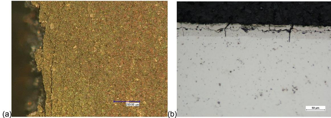
**Fig. 4.** A macro image of the side surface of the fatigue scrap, with visible cracks (a) and longitudinal fatigue scrap with the cracks in the aluminide layer (b)
