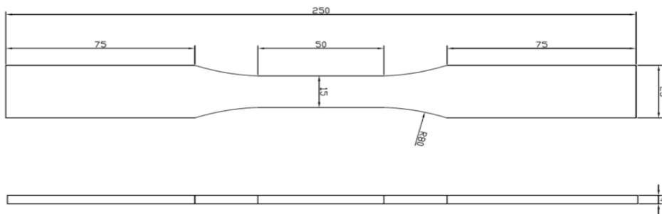
**Fig. 1.** The geometry of the sample used for deformation measurement
