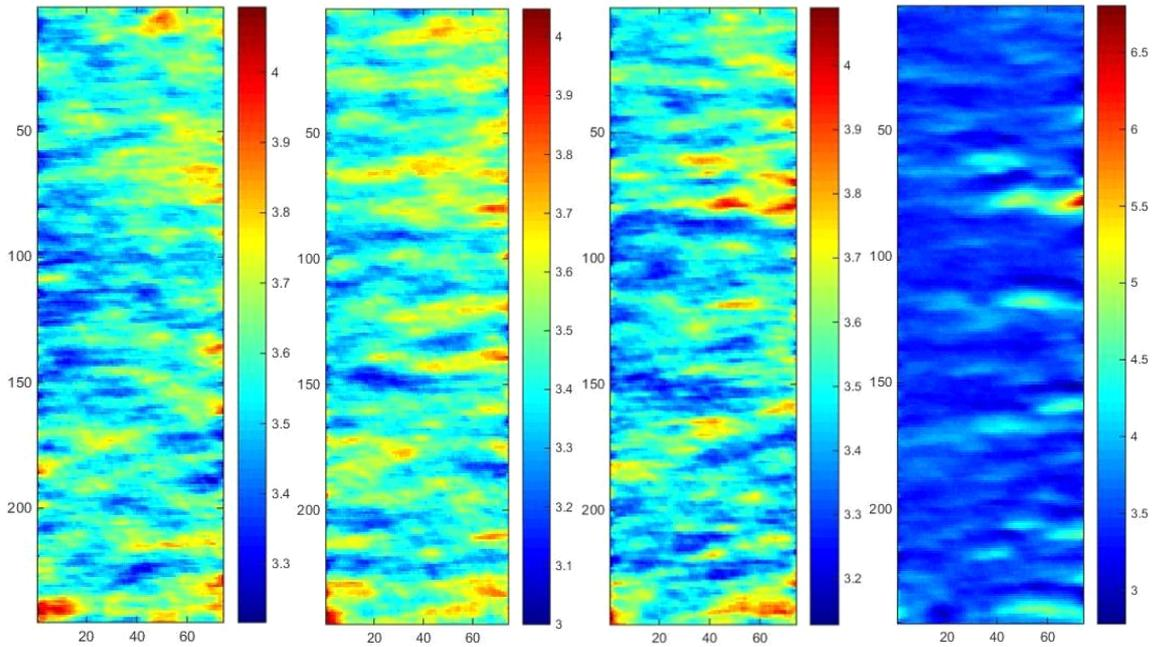
**Fig. 8.** Map of deformation in the selected load cycles (1k, 20k, 40k and 60k), amplitude 650 MPa, sample with layer 40  $\mu\text{m}$
