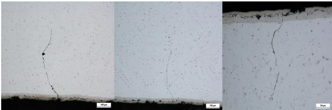
**Fig. 7.** Propagation of the cracks from layer to the matrix from nickel alloy
