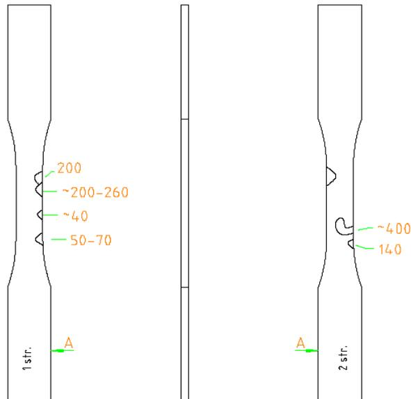
**Fig. 6.** Sample after 80 000 load cycles used in eddy currents measurements (draft)
