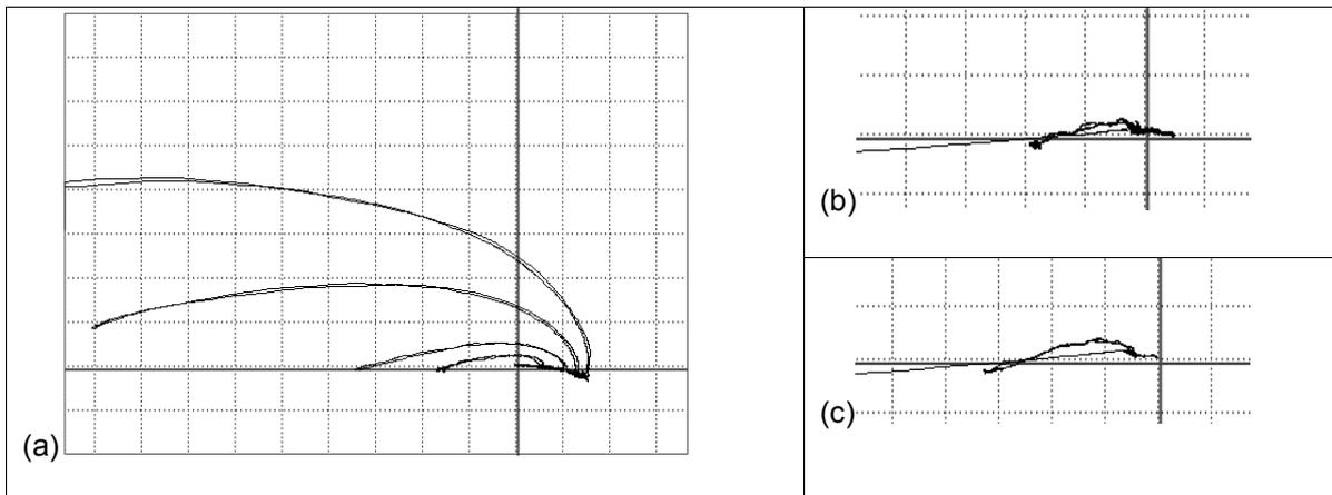
**Fig. 3.** Eddy current characteristics due to: discontinuities in the reference samples (a), a crack in the unloaded sample (b), a crack in the loaded sample (c)
