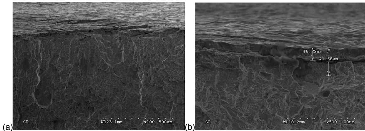
**Fig. 5.** Image of the fatigue fracture with the visible cracks in aluminide layer, obtained with the use of SEM
