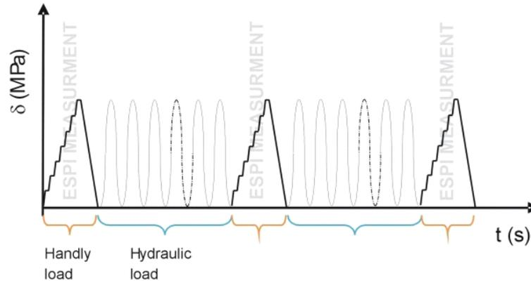
**Fig. 2.** Diagram of the sample loads and ESPI measurements
