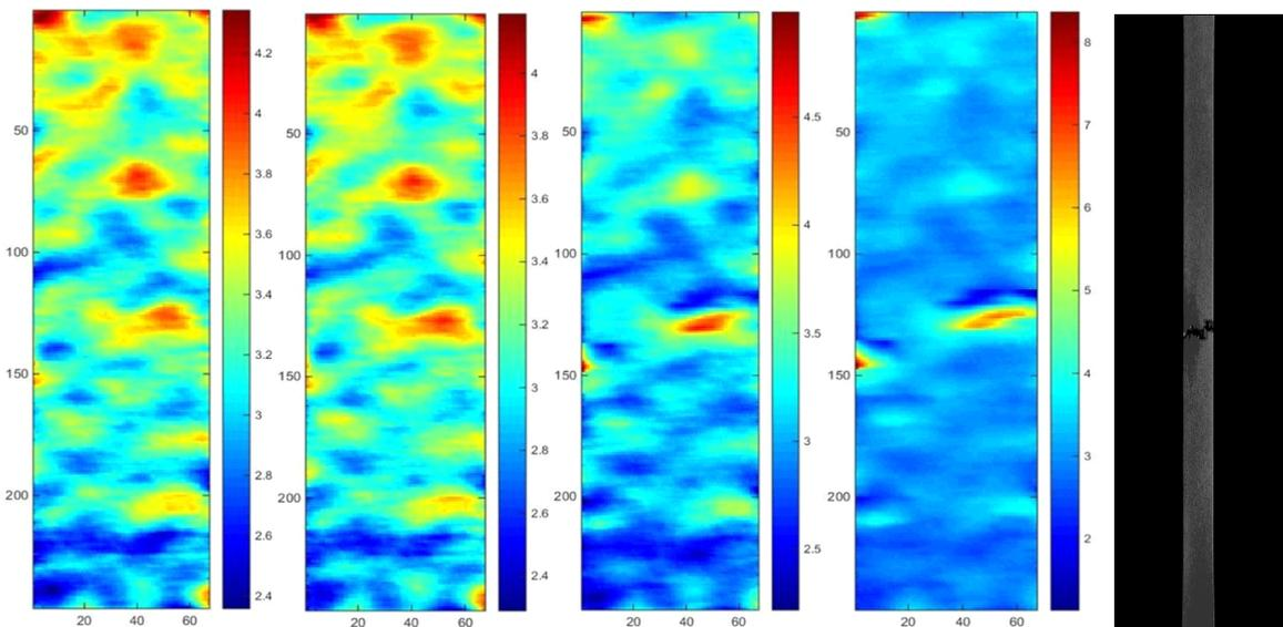
**Fig. 9.** Map of deformation in the selected load cycles (1k, 20k, 40k and 50k), amplitude 600 MPa, sample with layer 40  $\mu\text{m}$
