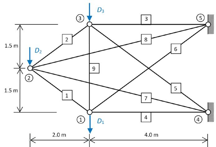
**Fig. 6** Planar 9-bar truss structure
