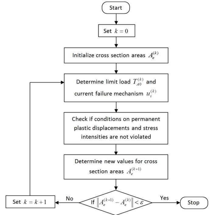
Fig. 3 Flow chart of the proposed algorithm.
