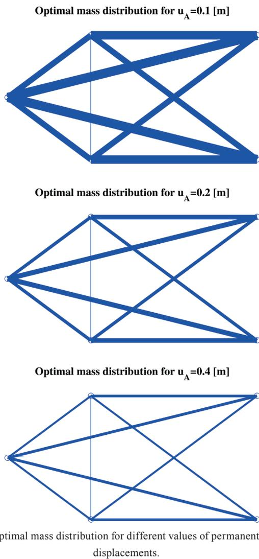
Fig. 8 Optimal mass distribution for different values of permanent plastic displacements.
