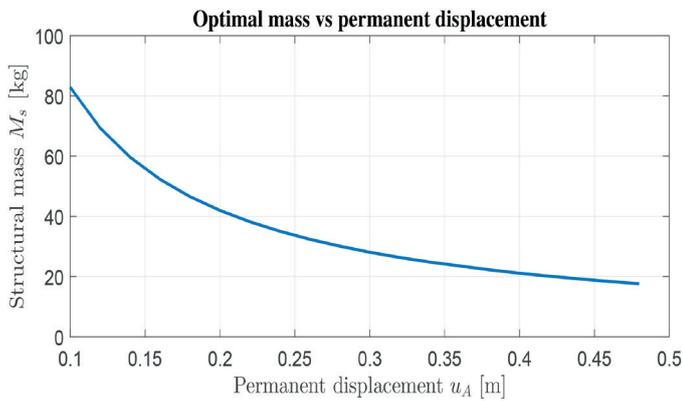
Fig. 7 Optimal solution as a function of allowable permanent plastic displacement.
