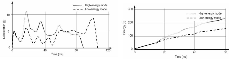
Figure 12: Impacting mass deceleration and dissipated energy versus time curves
