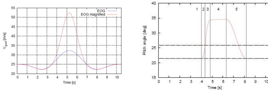
Figure 5: a) Extreme operating gust, b) Pitch angle changes in terms of control phases
