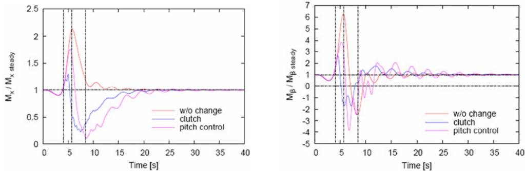
Figure 7: a) Tower bending moment, b) Blade bending moment
