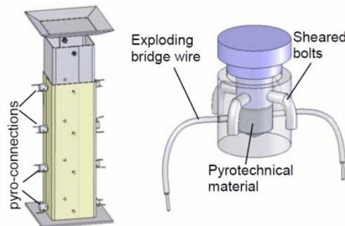
Figure 10: Pyrotechnical adaptive impact energy absorber
