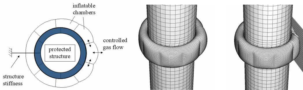
Figure 15: Inflatable structure protecting wind turbine tower: a) simplified 2D model, b) initial inflation before collision, c) deformation during impact
