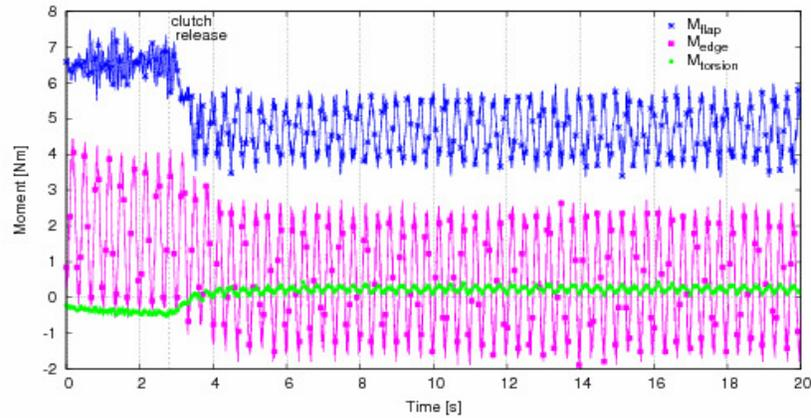
Figure 9. Reaction moments at root; rotor speed 180RPM.
