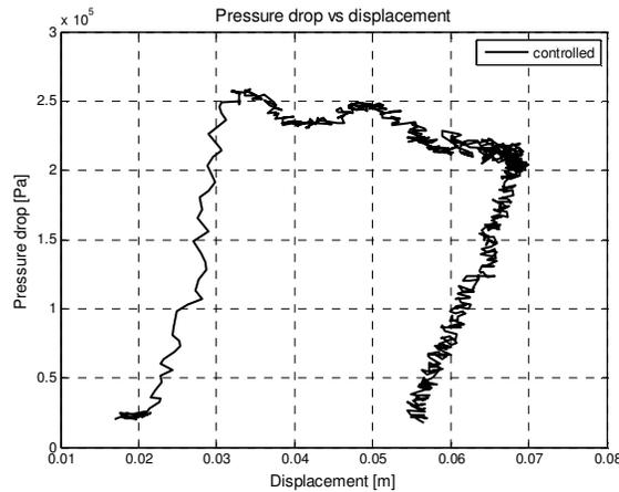
Figure 4: Pressure difference between two sides of the piston during the impact loading in the domain of the piston stroke.
