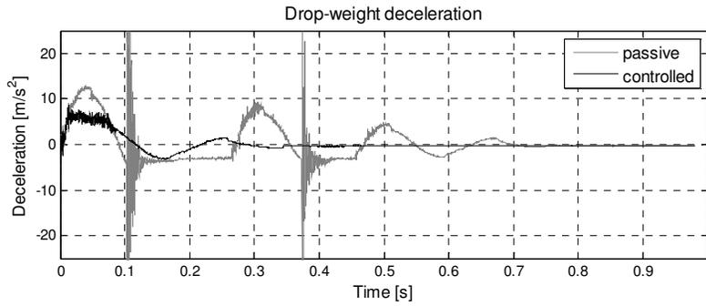
Figure 3b: Comparison of two modes of the absorber operation: passive and active.
