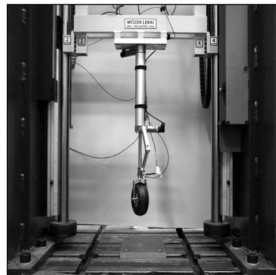
Figure 1: Pneumatic landing gear: a) operating principle, b) experimental stand
