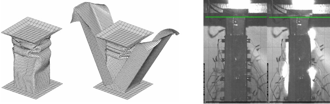
Figure 11: a) Passive (left) and active (right) modes; b) Experimental assessment: absorber before impact (left) and firing sequence (right)
