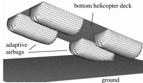
Figure 17: Numerical simulation of emergency landing with adaptive airbags
