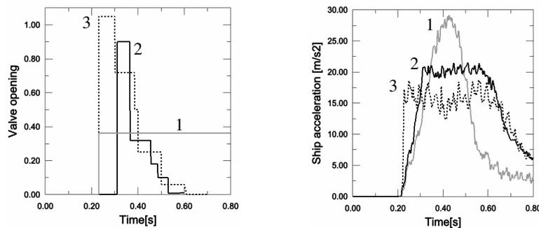
Figure 16: Strategies of acceleration mitigation: 1) constant valve opening, 2) pressure only released during impact, 3) additional inflation at the beginning of impact
