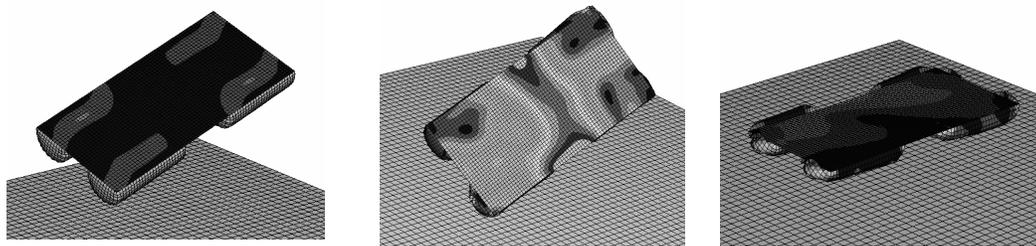
Figure 19: a) Considered landing scenario, b) non-optimal passive response with rear part rebound, c) optimal uniform airbags compression obtained by semi-active pressure control
