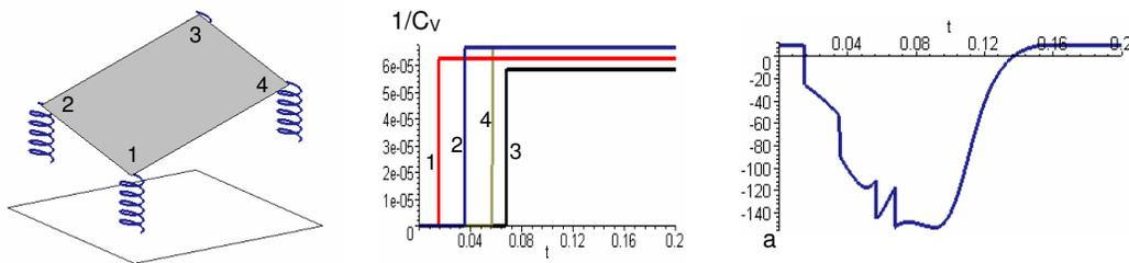
Figure 18: a) Simplified model of emergency landing, b) applied valve opening (represented by inverse of flow coefficient), c) resulting linear acceleration of the center of the mass
