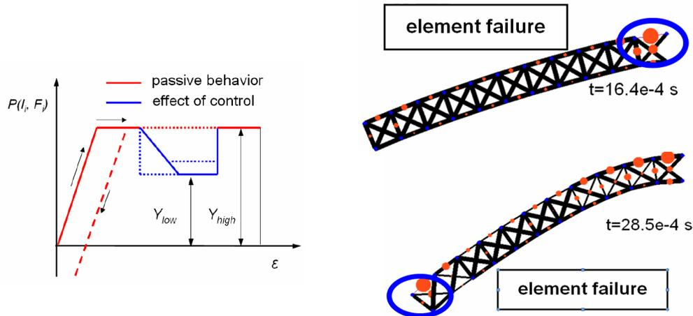
Figure 14: a) Elasto-plastic characteristic of the truss element with modifications due to control function; b) Terminal states (at the failure moment of first element) for the passive structure (left) and self controlled structure (right)
