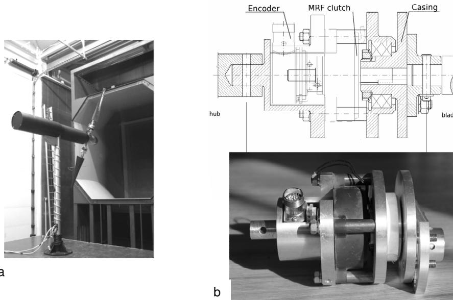
Figure 8. a) Experimental set-up in wind tunnel; b) Adaptive clutch (cross section and general view)
