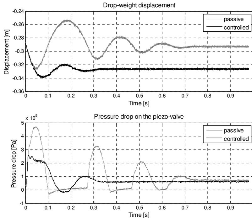
Figure 3a: Comparison of two modes of the absorber operation: passive and active.
