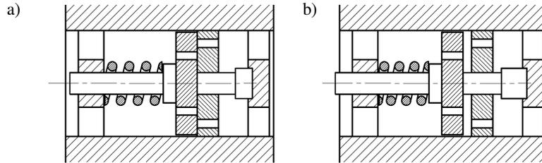
Figure 2: Cross-sectional view through the valve: a) closed, b) opened.
