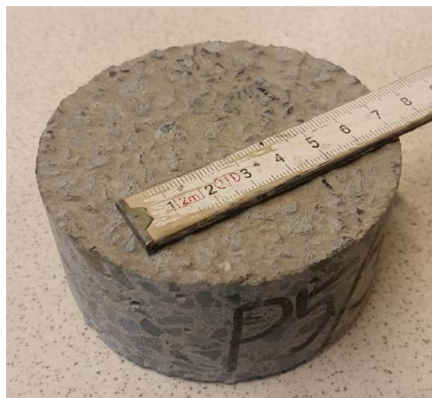
Fig. 4. Drilled concrete core from EAC slab
