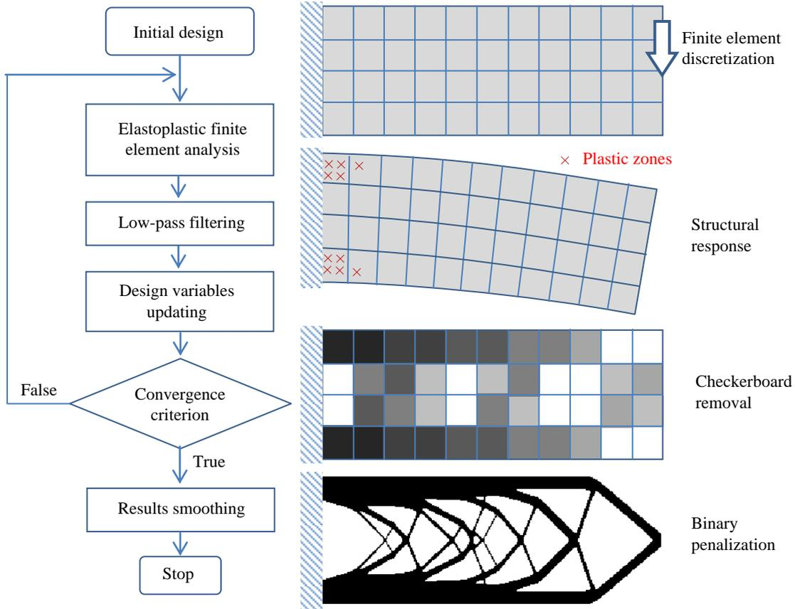
Fig 1. Computational steps in structural topology optimization
