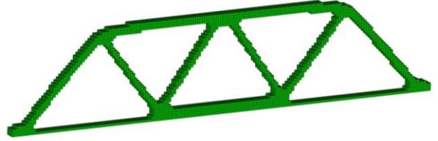
Fig.3. Optimal topology for load equal to 0.5 x collapse load.
