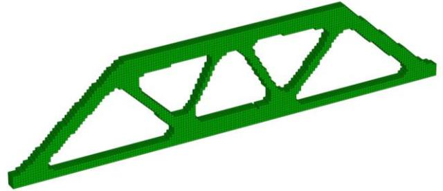
Fig.4. Optimal topology for load equal to 0.95 x collapse load.
