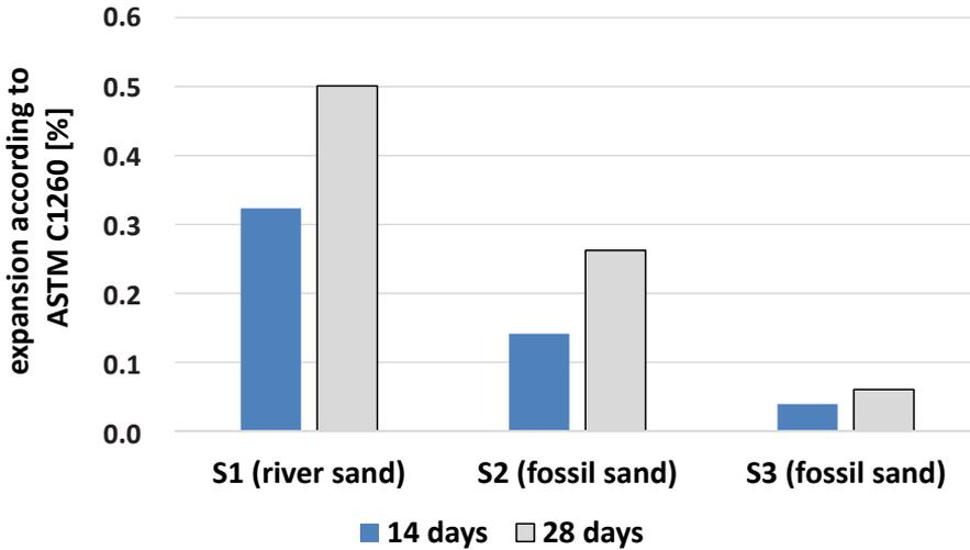
Figure 5. The results of sand mortar-bar expansion according to ASTM C1260 after 14 and 28 days of exposure in 1 M NaOH in 80°C
