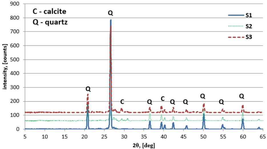
Figure 4. X-ray diffraction (XRD) patterns with main characteristic peaks in the tested sands
