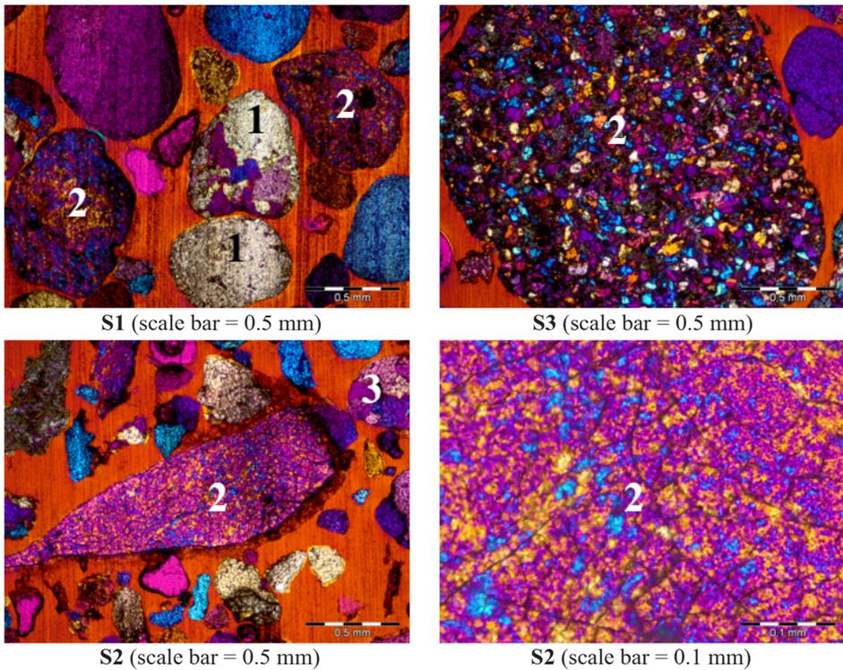
Figure 2. Sections of micro- and cryptocrystalline form of quartz (fine grained chert), (S1-S3), 1 – monomineral quartz, 2 – fine grained chert, 3 – granitic rock
