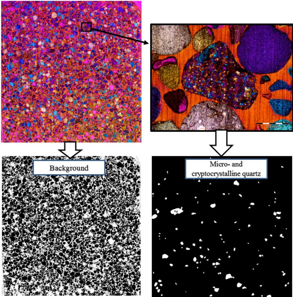
Figure 3. Scheme of the image analysis procedure of the micro- and cryptocrystalline quartz estimation
