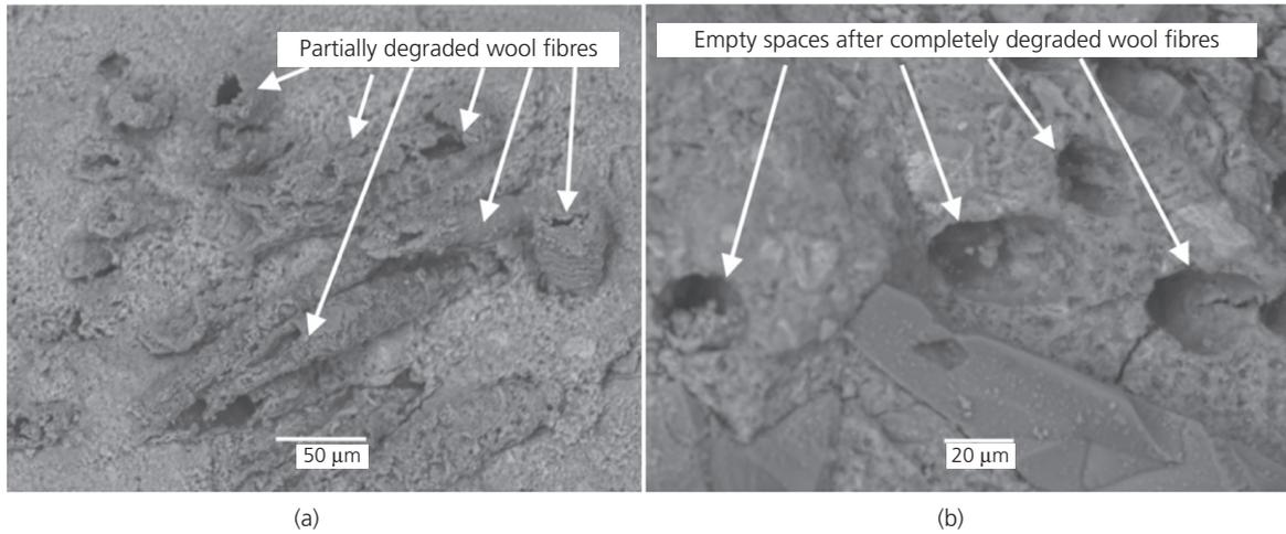
Figure 9. Microstructure of specimens made with high-alkali cement and addition of wool fibres after: (a) 3 days of curing in water at 20°C; (b) 27 days of curing in water at 20°C
