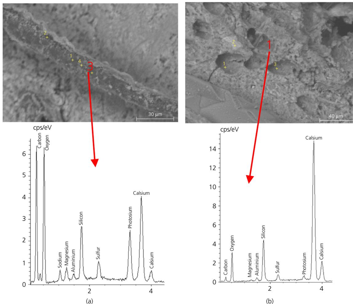
**Figure 7.** Microstructure of specimens made with high-alkali cement and reinforced with wool fibres with EDX analysis in microareas: (a) H\_4 – after 3 days of curing in water at 20°C (analysis in the microarea on wool fiber); (b) H\_3 – after 27 days of curing in water at 20°C (microarea analysis in a matrix after a degraded wool fiber)
