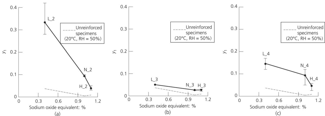
**Figure 8.** Residual stress  $y_1$  measured in the three-point bending tests: (a) specimens cured for 27 days in room conditions (20°C, RH = 50%); (b) specimens cured for 27 days in water (20°C); (c) specimens cured for 3 days in water (20°C)
