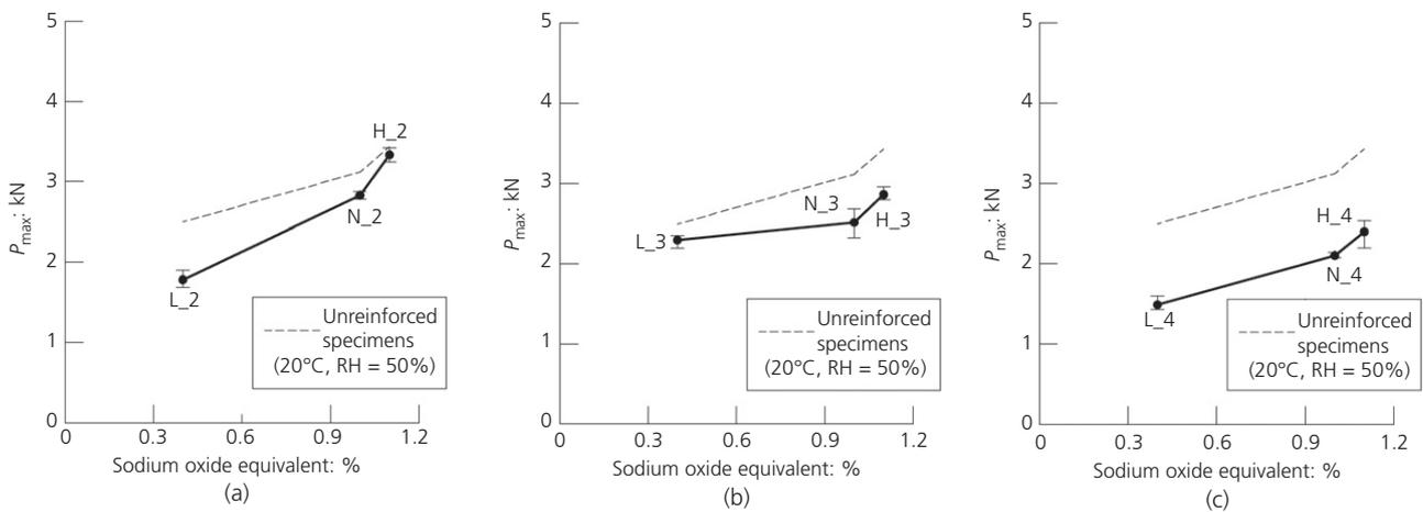
Figure 5. Flexural strength  $P_{max}$  measured in the three-point bending tests: (a) specimens cured for 27 days in room conditions (20°C, RH = 50%); (b) specimens cured for 27 days in water (20°C); (c) specimens cured for 3 days in water (20°C)
