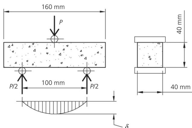
**Figure 2.** Three-point bending tests for cementitious mortars (BSI, 2005)
