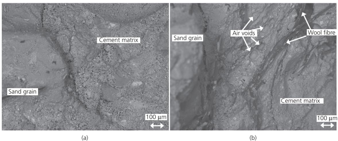
Figure 6. Microstructure of specimens made with low-alkali cement after 27 days of curing in 20°C and 50% RH (scale bar – 100 μm): (a) reference specimen L\_1; (b) specimen with addition of wool fibres L\_2
