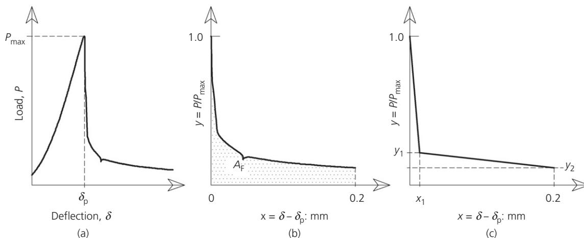
Figure 3. Results of three-point bending tests: (a) whole  $P-\delta$  diagram; (b) post-peak behaviour; (c) bilinear relationship used to quantify the effect of fibres
