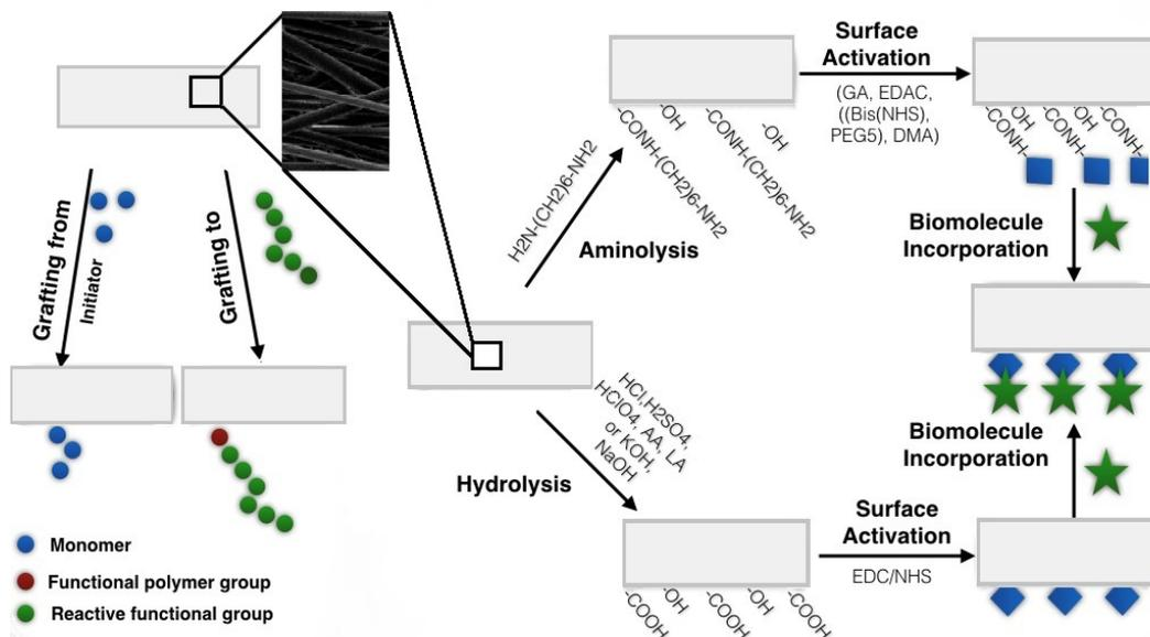
Figure 1. Chemical functionalization of electrospun nanofibers.
