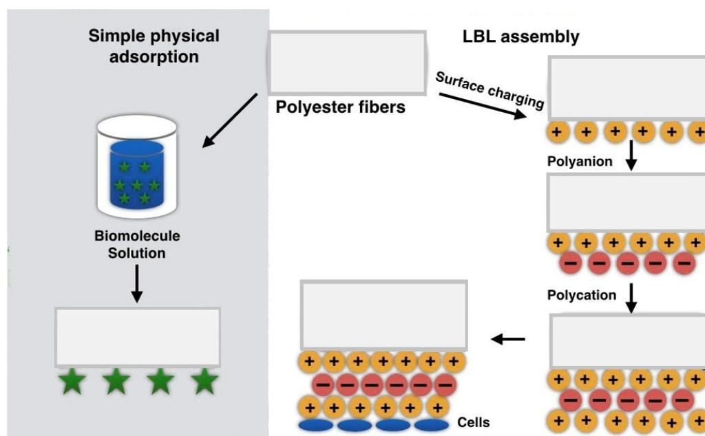
Figure 3. Physical functionalization of electrospun nanofibers.
