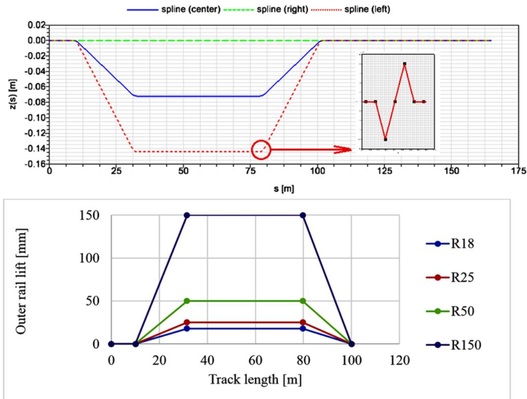
Fig. 9. A novel geometry of test track for proposed research methodology
