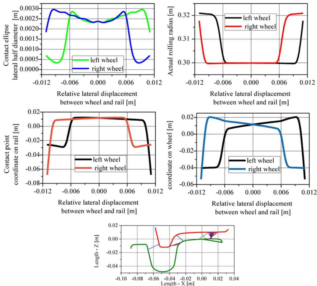
Fig. 6. Mutual positions of the wheel-rail profiles of the IRW tram with the PST wheel profile and the Ri60N rail profile with equivalent conicity of  $\lambda = 0.013$  and lateral displacement of 3 mm
