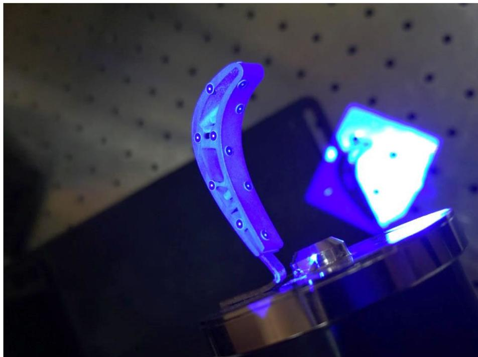
**Figure 6.** The turbine blade section during the digitization process.
