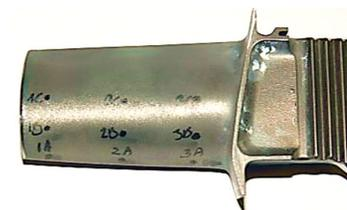
**Figure 2.** Places of impedance phase angle measurement.
