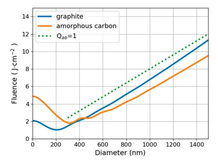
**Figure 1.** Threshold fluence necessary for the evaporation of spherical carbon particles in water by a laser beam with a wavelength of 1064 nm.
