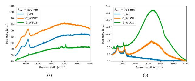
**Figure 8.** Raman spectra of Samples B\_W1, C\_W1W2, and B\_W1U2 excited at (**a**) 532 nm (the B\_W1U2 signal was multiplied by 2) and (**b**) 785 nm (the B\_W1U2 signal was divided by 5).
