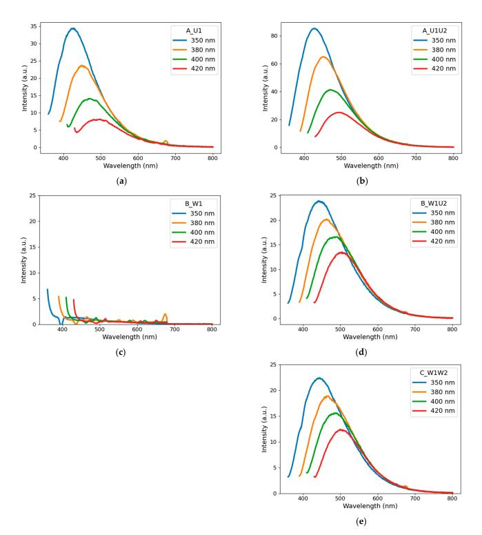
**Figure 3.** Photoluminescence spectra of carbon nanostructures obtained via Approaches (**a**) A\_U1, (**b**) A\_U1U2, (**c**) B\_W1, (**d**) B\_W1U2, and (**e**) C\_W1W2. Excitation wavelengths ranged from 350 to 420 nm.
