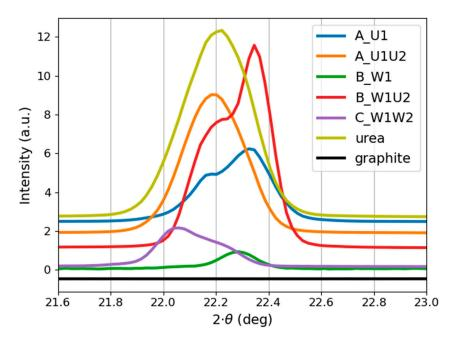
**Figure 7.** Comparison of 22° peak appearance for the carbon nanostructures, urea solution, and graphite target. The B\_W1 signal was multiplied by 10.
