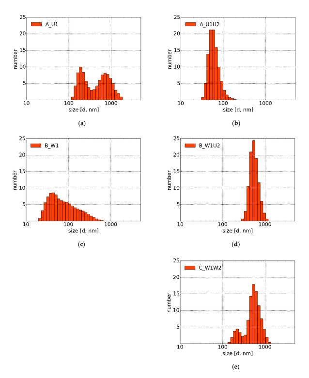
**Figure 5.** Size distributions of Samples (**a**) A\_U1, (**b**) A\_U1U2, (**c**) B\_W1, (**d**) B\_W1U2, and (**e**) C\_W1W2. The mean standard deviation for all presented graphs was less than 9%.
