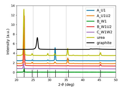
**Figure 6.** Diffraction patterns of the carbon nanostructures, reference sample (urea solution), and graphite target. The B\_W1 signal was multiplied by 10. Peak positions are indicated by black vertical lines.
