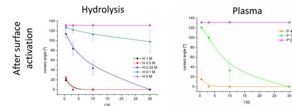
Up: Graphs showing a decrease in water contact angle due to surface activation with NaOH and plasma in function of a drop contact time with the material (0.2 - 30 s). No change was observed for samples after aminolysis (PLCL=131,43°).
