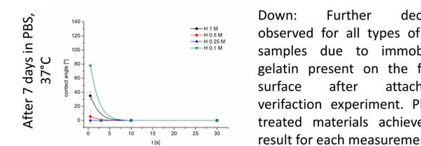
Down: Further decrease observed for all types of the samples due to immobilized gelatin present on the fibres' surface after attachment verification experiment. Plasma treated materials achieved 0° result for each measurement.
