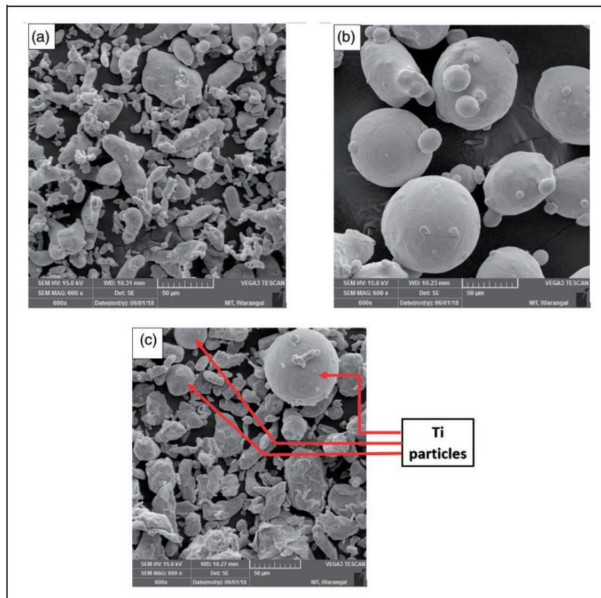
**Figure 1.** Scanning electron microscope picture of pure powder particles (a) Al. (b) Ti and (c) Blended Al - Ti.
