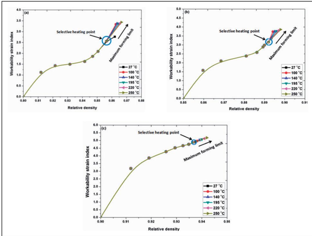
**Figure 12.**  $\beta_c$  of selective heated porous Al – 4% Ti samples concerning relative density for various preforms IRDs (a) 80%. (b) 85% and (c) 90%.
