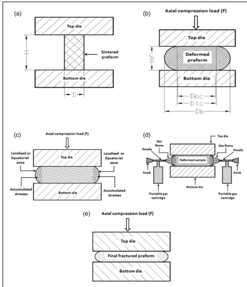
**Figure 5.** The schematic diagram for conducting the SH upsetting test (a) Application of deformation load on the sintered specimen. (b) The specimen is deformed after the application of load. (c) Accumulation of stresses in the equatorial position of the deformed sample. (d) Adopting the SH technique in the outer region of the deformed sample and (e) Application of load on the deformed samples after the SH.
