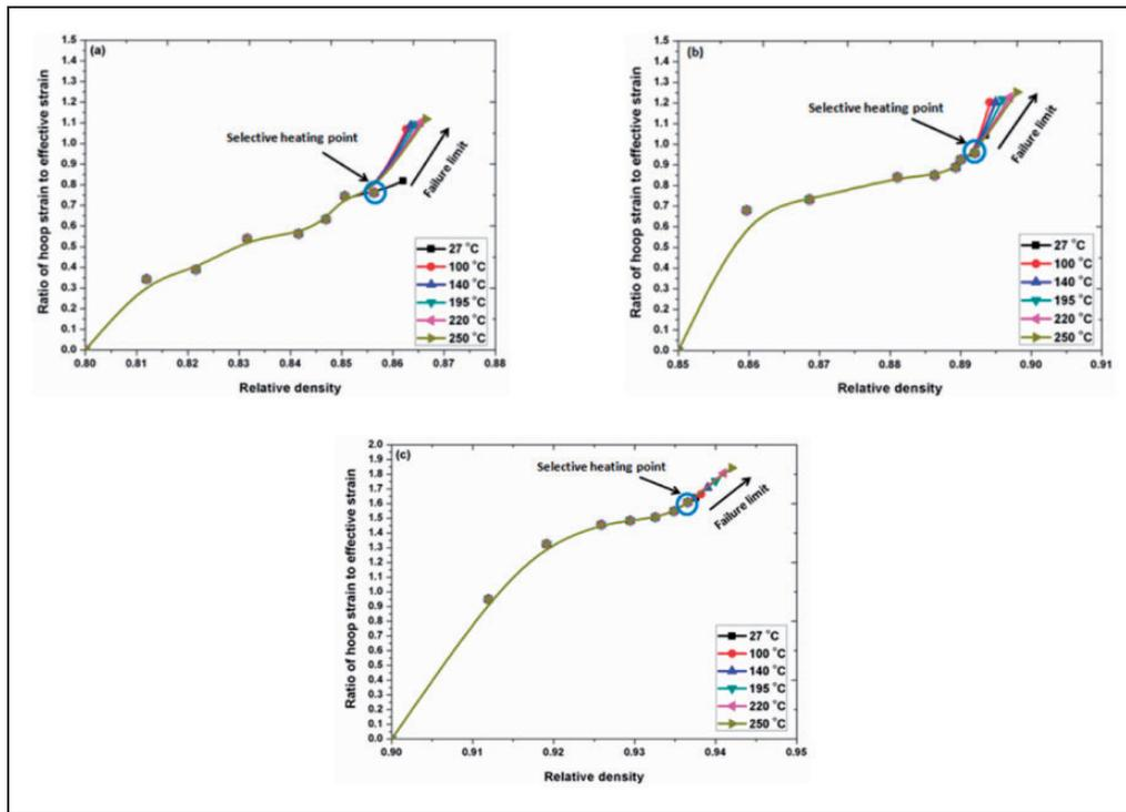
**Figure 14.**  $\varepsilon_{\theta}/\varepsilon_{eff}$  plot of selective heated P/M Al – 4% Ti samples concerning relative density for several IRDs (a) 80%. (b) 85% and (c) 90%.
