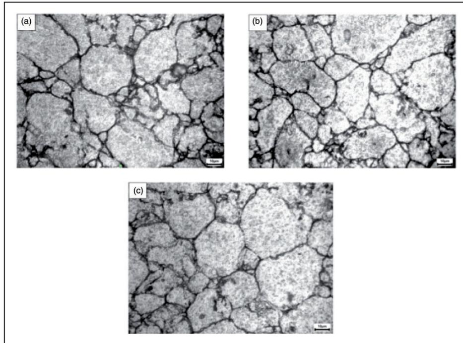
**Figure 15.** Microstructure image of P/M Al – 4% Ti samples in the sintered condition at several IRDs (a) 80%. (b) 85% and (c) 90%.
