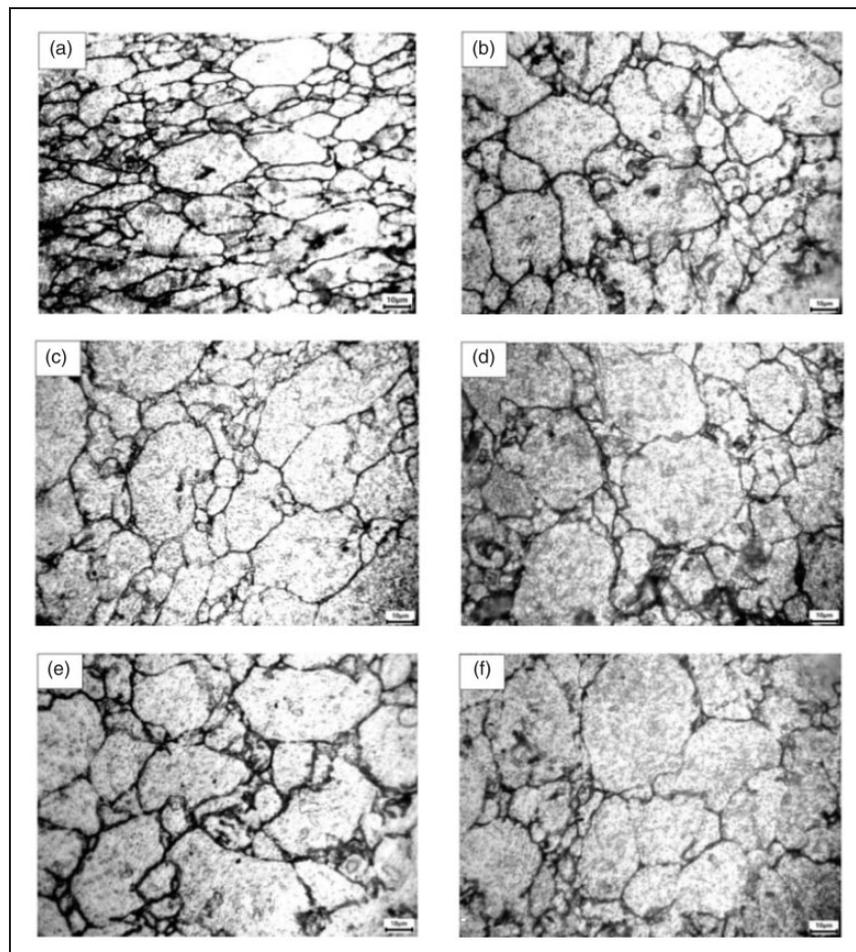
**Figure 16.** Optical micrograph of compressed porous Al – 4% Ti sample for various SH in °C (a) 27, (b) 100, (c) 140, (d) 195, (e) 220 and (f) 250.
