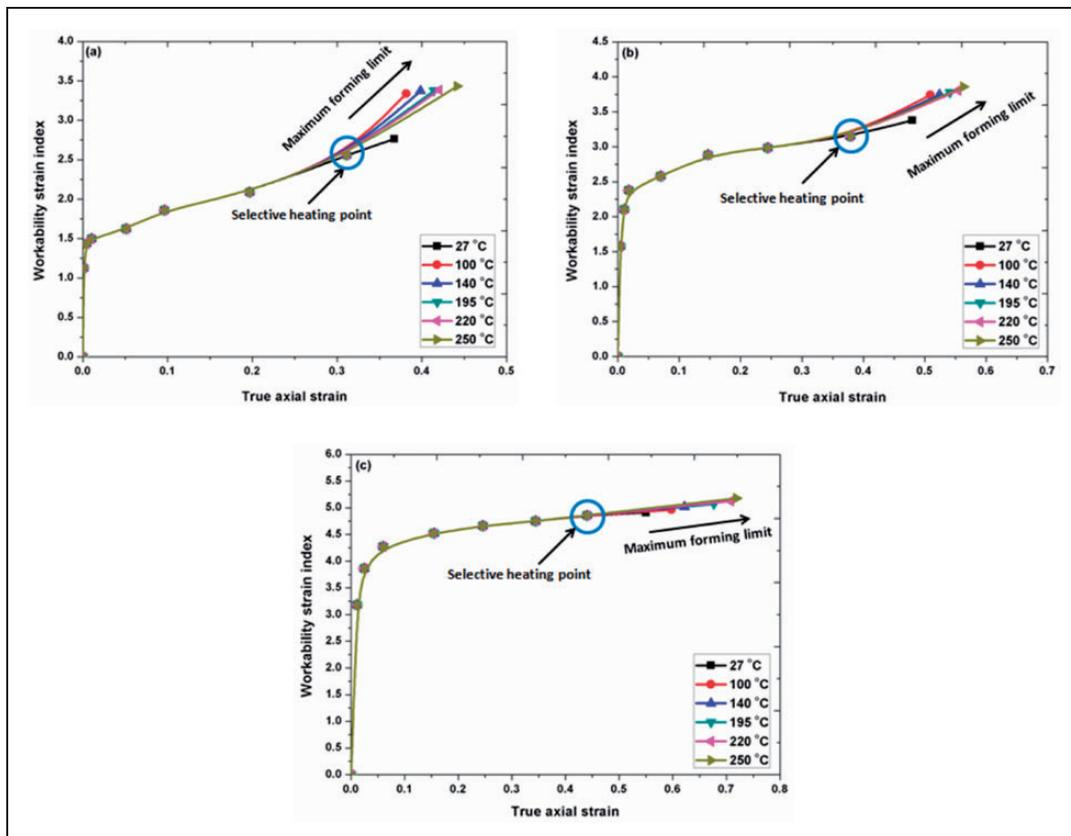
Figure 9.  $\beta_{\epsilon}$  of selective heated P/M Al – 4% Ti samples concerning  $\epsilon_z$  for various preforms IRDs (a) 80%. (b) 85% and (c) 90%.
