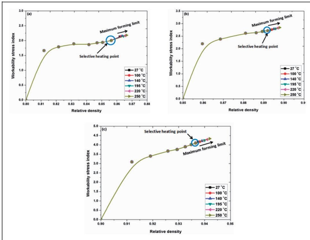
**Figure 10.**  $\beta_\sigma$  of selective heated porous Al – 4% Ti samples concerning relative density for various preforms IRDs (a) 80%. (b) 85% and (c) 90%.
