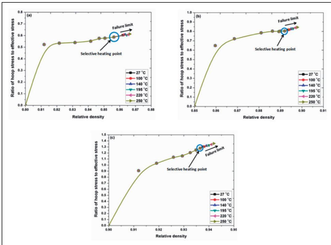
**Figure 13.**  $\sigma_\theta/\sigma_{eff}$  plot of selective heated P/M Al – 4% Ti samples concerning relative density for several IRDs (a) 80%. (b) 85% and (c) 90%.
