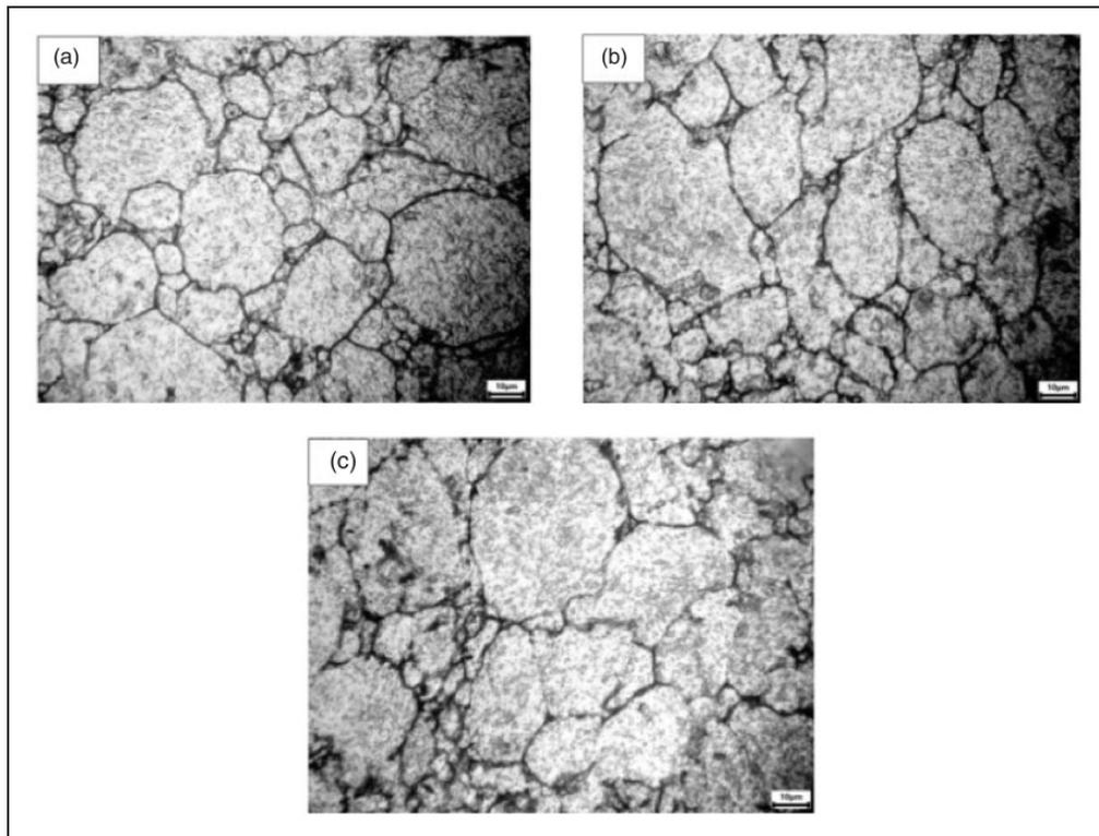
**Figure 17.** Microstructure of forged porous Al – 4% Ti sample at the SH of 250 °C for several IRDs (a) 80%, (b) 85% and (c) 90%.
