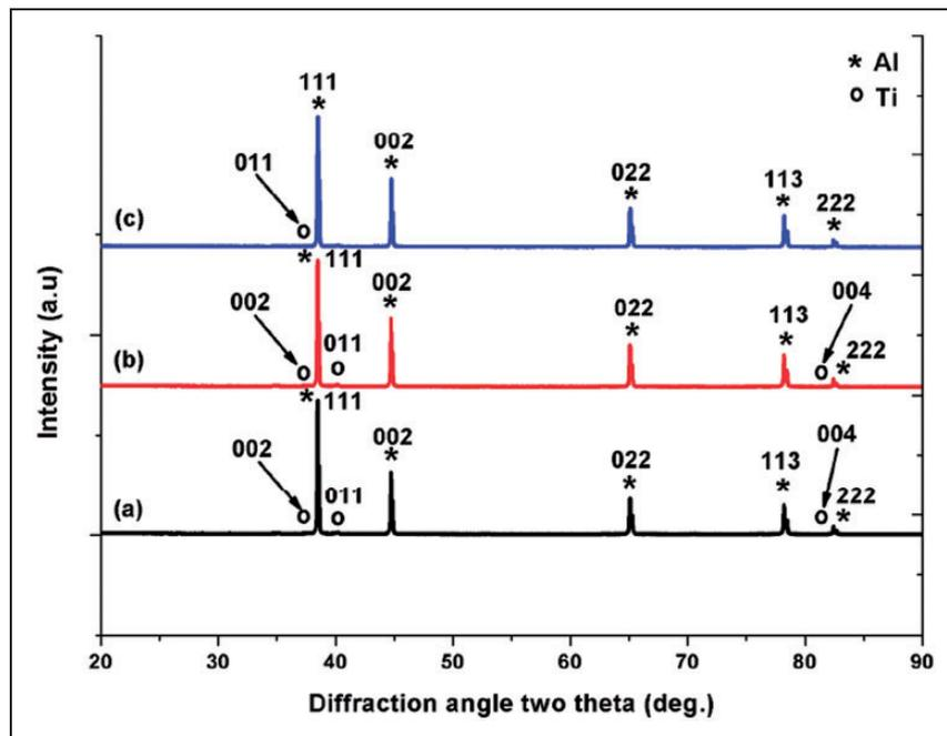
Figure 2. X-ray diffraction plot of sintered P/M Al – 4% Ti samples for several IRDs (a) 80%. (b) 85% and (c) 90%.
