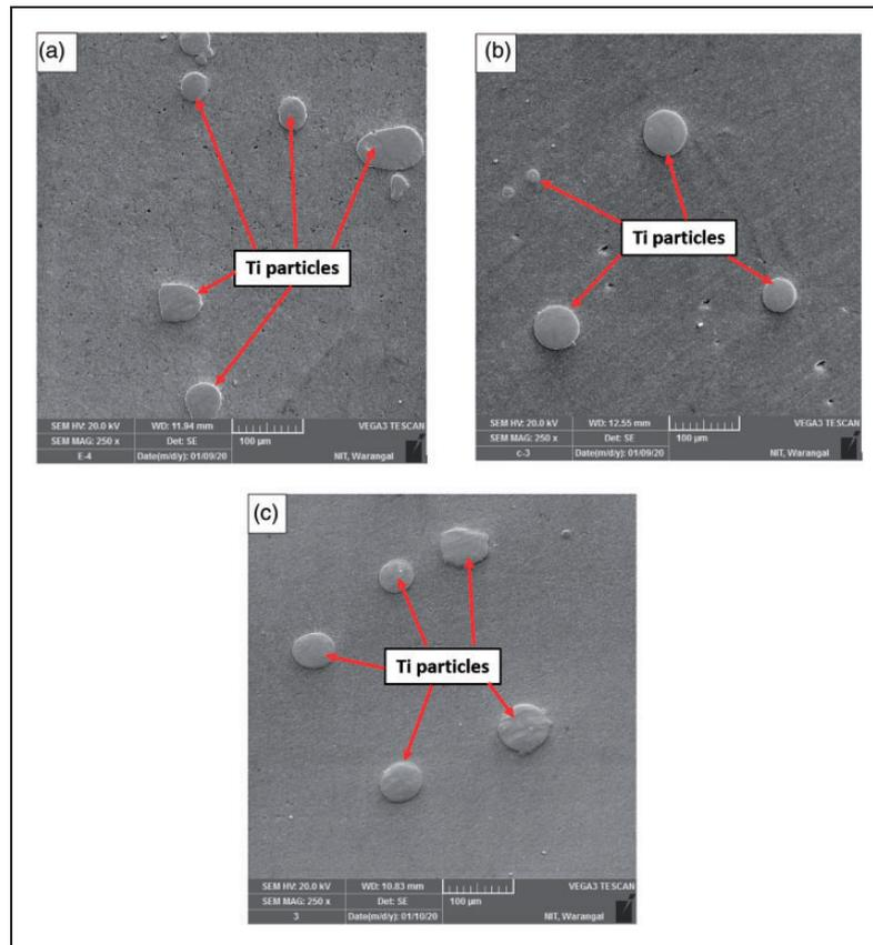
**Figure 3.** Scanning electron microscope image of sintered P/M Al – 4% Ti samples for several IRDs (a) 80%. (b) 85% and (c) 90%.
