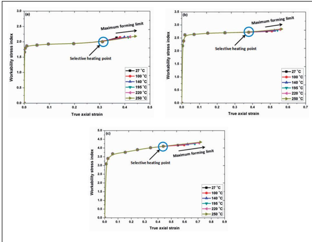
Figure 8.  $\beta_{\sigma}$  of selective heated P/M Al – 4% Ti samples concerning  $\epsilon_z$  for various preforms IRDs (a) 80%. (b) 85% and (c) 90%.
