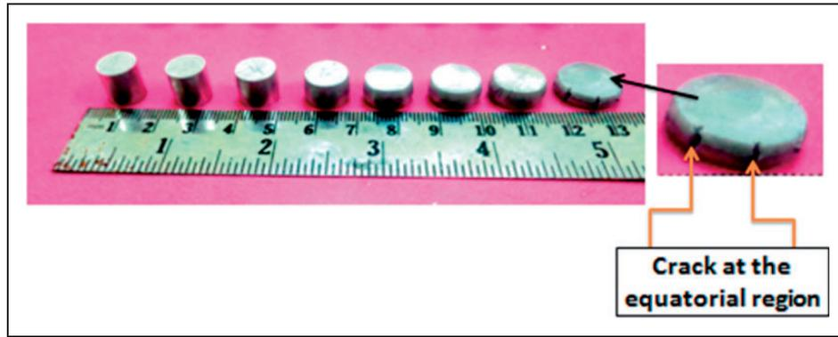
**Figure 6.** Actual P/M Al – 4% Ti components after the incremental deformation.
