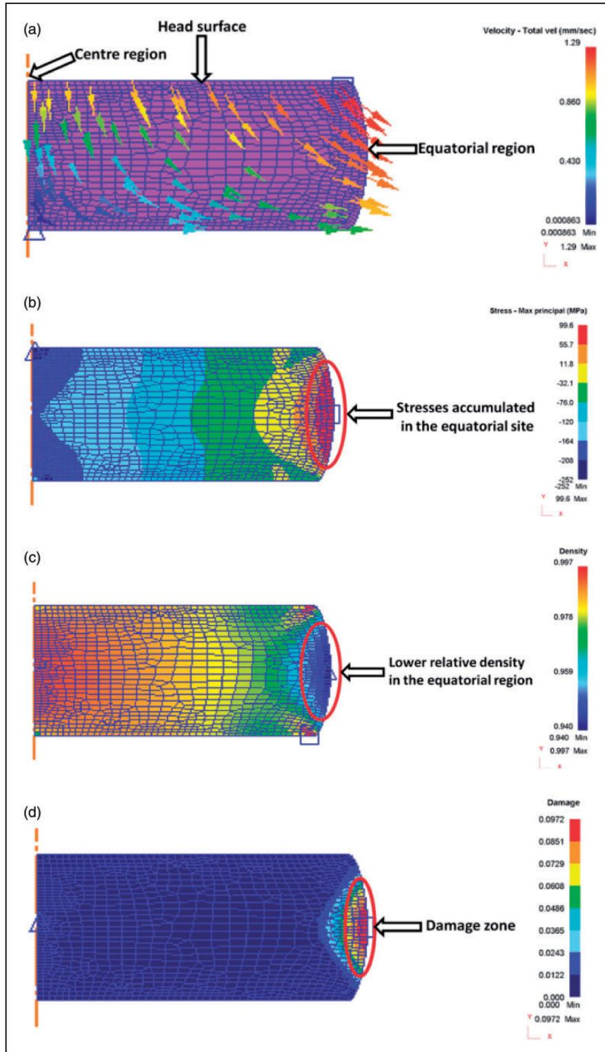
**Figure 7.** Finite element contour picture of forged P/M Al – 4% Ti samples (a) Velocity. (b) Stress. (c) Relative density and (c) Damage.
