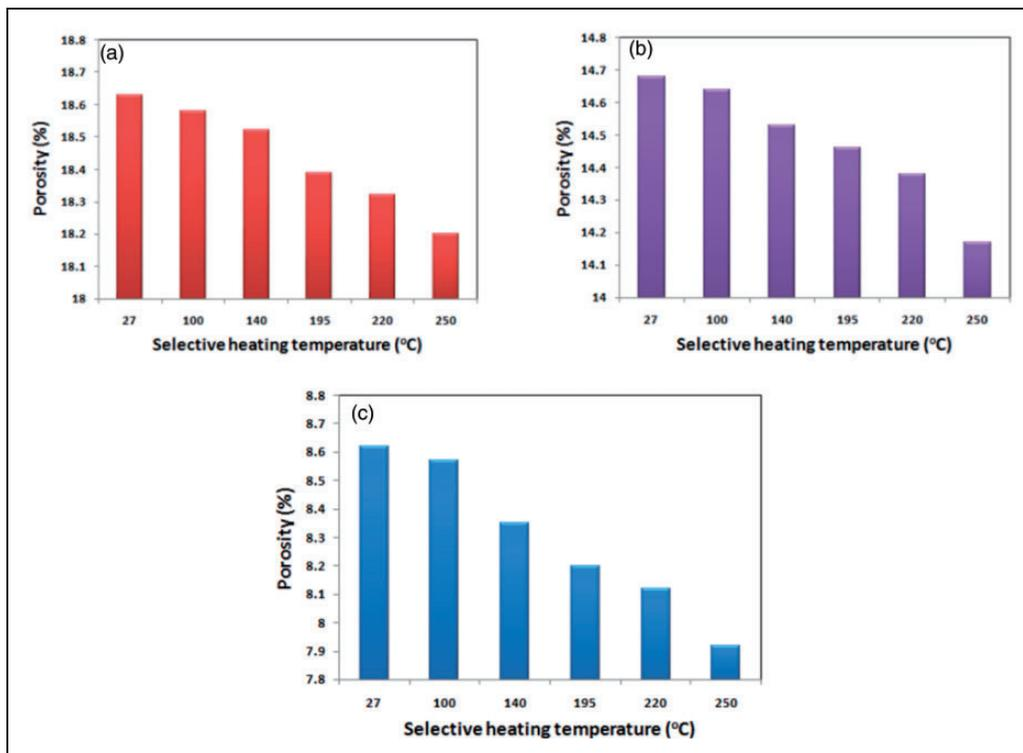
Figure 11. Porosity of the compressed selective heated Al - 4% Ti samples for several IRDs (a) 80%. (b) 85% and (c) 90%.
