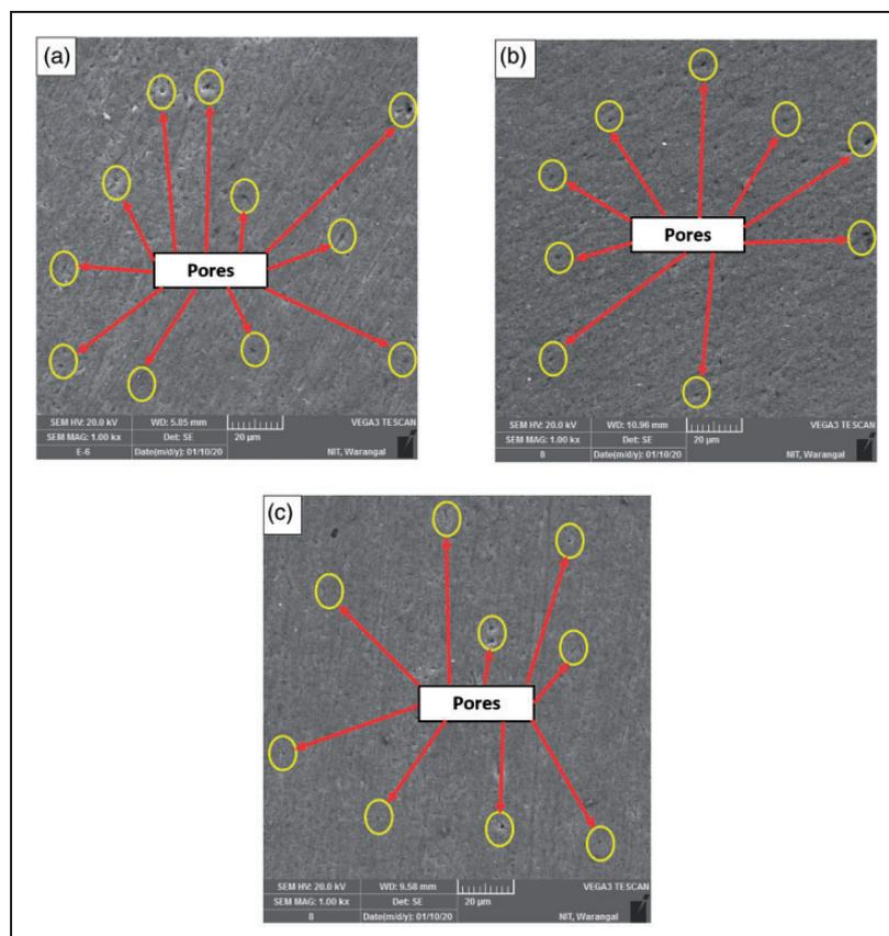
**Figure 4.** Microstructure of newly developed sintered P/M Al – 4% Ti samples for several IRDs (a) 80%. (b) 85% and (c) 90%.
